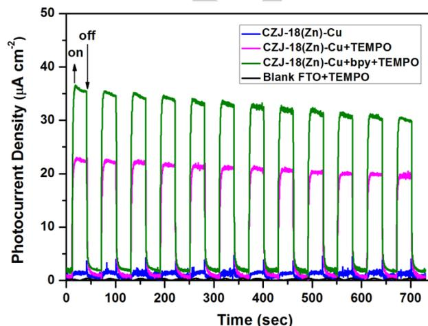
**Figure 3.** Transient photocurrent responses of CZJ-18(Zn)-Cu in 0.1 M  $\text{Bu}_4\text{NClO}_4$  acetonitrile solution at a bias of 0 V (vs. SCE electrode) at room temperature under a 300 W Xenon lamp irradiation with a 400 nm light cut-off filter.
