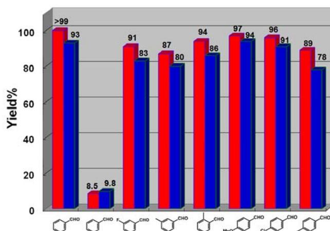
**Figure 2.** The yields of aldehydes catalyzed by CZJ-18(Cu)-Cu at 65 °C for 16 h (red columns) and CZJ-18(Zn)-Cu at room temperature for 10 h irradiated by visible light (blue columns). The numbers on the top of the columns are the yields of aldehydes. The third and fourth columns are the results catalyzed by  $\text{Cu}-\text{Me}_8\text{OCPP}/\text{Cu}(\text{ClO}_4)_2$  and  $\text{Zn}-\text{Me}_8\text{OCPP}/\text{Cu}(\text{ClO}_4)_2$ , respectively.
