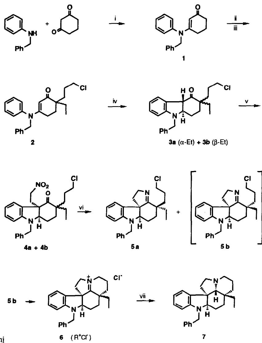
**Reagents and conditions :** i) toluene,  $\Delta$ , 15h; ii) LDA,  $C_2H_5I$ , THF, -78°C; iii) LDA,  $I(CH_2)_3Cl$ , THF, -78°C; iv)  $h\nu$ , benzene, argon, 0,5 h ; v) LDA, nitroethylene, THF, -78°C ; vi)  $HCOONH_4$ , 10 % Pd/C, MeOH, 65 °C, 15 h; vii)  $H_2$ , 5 %  $Pt/Al_2O_3$ , EtOH, 3 atm., room temperature, 48 h.
