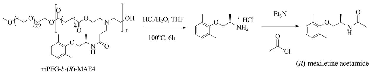
**SCHEME 2** Hydrolysis of mPEG-*b*-(*R*)-MAE4 and synthesis of (*R*)-mexiletine acetamide.
