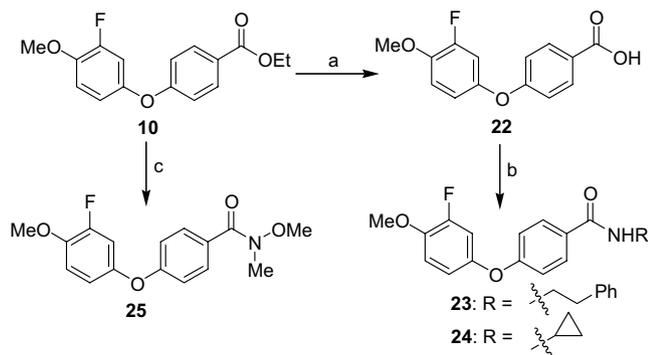
**Scheme 2.** Reagents: (a) LiOH, H<sub>2</sub>O–THF, 86%; (b) phenethylamine, DCC, DMAP, THF, 53% for **23**; cyclopropylamine, DCC, DMAP, THF, 77% for **24**; (c) Me(MeO)NH · HCl, *i*-PrMgCl, THF, 63%.
