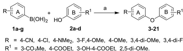
**Scheme 1.** Reagents and condition: (a) Cu(OAc)<sub>2</sub>, Et<sub>3</sub>N, CH<sub>2</sub>Cl<sub>2</sub>, rt 42–84%.
