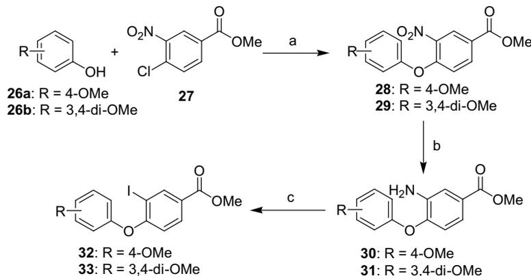
**Scheme 3.** Reagents and conditions: (a) aq KOH, reflux, 76–88%; (b) Pd/C, H<sub>2</sub>AcOH, rt; (c) (i) NaNO<sub>2</sub>, concd H<sub>2</sub>SO<sub>4</sub>, 0–5 °C; (ii) KI, H<sub>2</sub>O, rt–70 °C, 55–71% for two steps.
