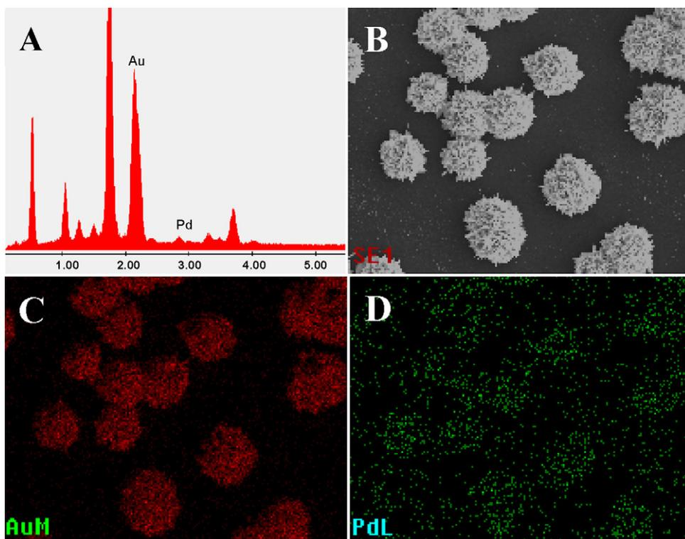
Fig. 5. (A) EDX analysis in a selected domain of ultrathin Pd coated HFGMs sample, (B) the morphological image of the as-prepared sample and X-ray maps of Au (C) and Pd (D), respectively, corresponding to (B).
