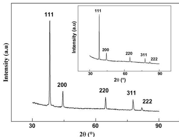
Fig. 7. XRD pattern of ultrathin Pt coated HFGMs sample. The inset is XRD pattern of the HFGMs sample.
