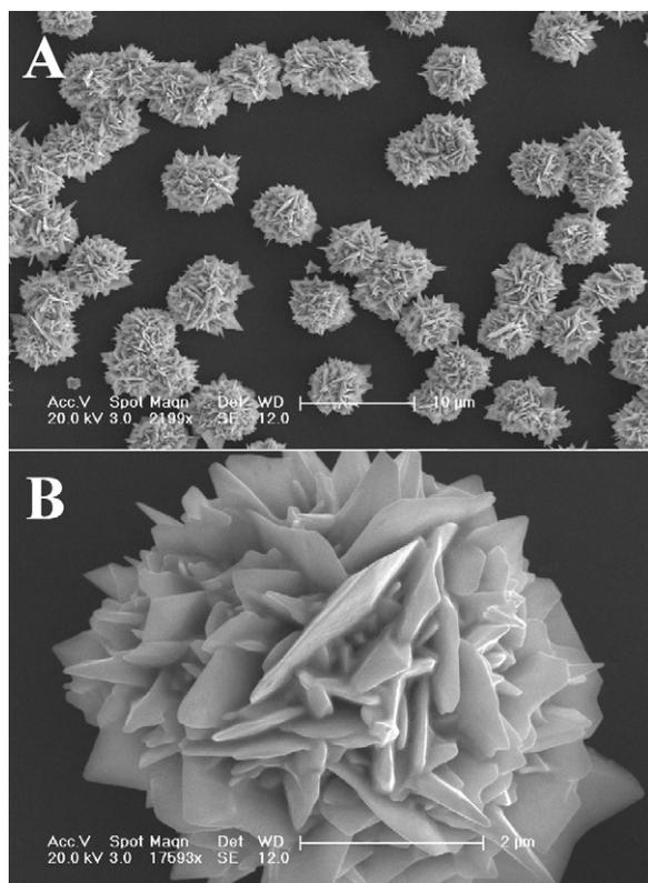
Fig. 1. Typical FE-SEM images of the HFGMs located at ITO substrate at different magnifications. The scale bar is 10 and 2  $\mu\text{m}$  for (A) and (B), respectively.
