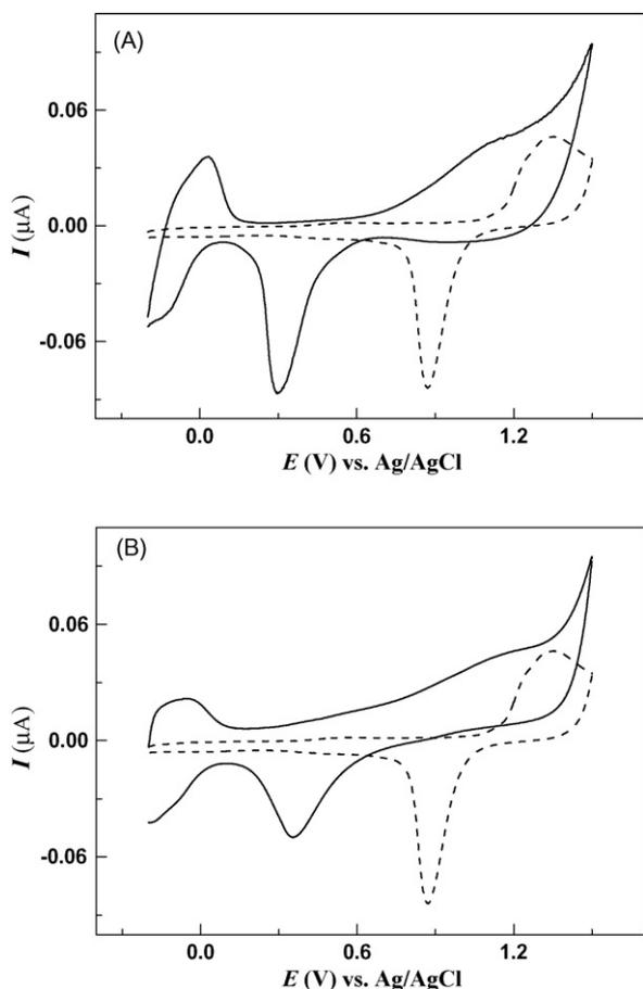
Fig. 3. Cyclic voltammograms for HFGMs modified ITO substrates in deaerated 0.1 M  $\text{H}_2\text{SO}_4$  before (dash trace) and after (solid trace) coating with ultrathin Pd (A) and Pt (B). Scan rate is  $50 \text{ mV s}^{-1}$ .
