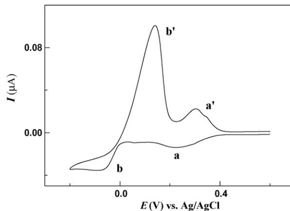
Fig. 2. Cyclic voltammograms for HFGMs modified ITO substrate in deaerated  $1 \text{ mM CuSO}_4 + 0.1 \text{ M H}_2\text{SO}_4$ . Scan rate is  $50 \text{ mV s}^{-1}$ .
