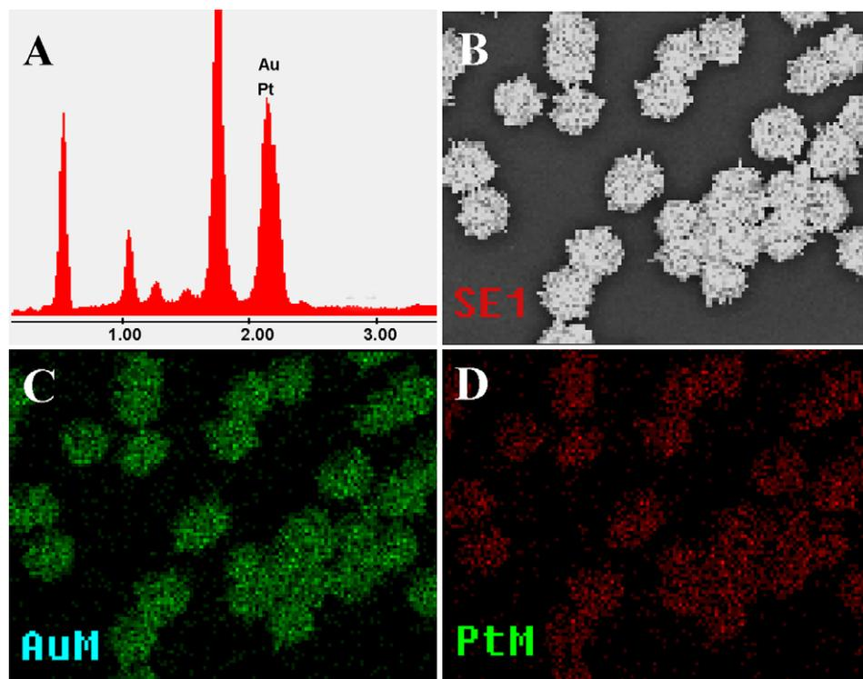
Fig. 6. (A) EDX analysis in a selected domain of ultrathin Pt coated HFGMs sample, (B) the morphological image of the as-prepared sample and X-ray maps of Au (C) and Pt (D), respectively, corresponding to (B).
