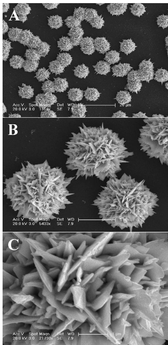
Fig. 4. Typical FE-SEM images of ultrathin Pd coated HFGMs located at ITO substrate at different magnifications. The scale bar is 20, 5 and  $1 \mu\text{m}$  for (A), (B) and (C), respectively.
