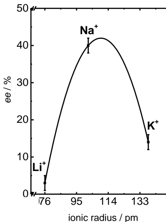
**Figure 6.** Effect of different alkali ions used for the functionalization of Pt NPs with PRO on the stereoselectivity. The solid line is a fit of the experimental data that serve merely as a guide to the eye. The ionic radii were taken from the literature.<sup>[35]</sup>
