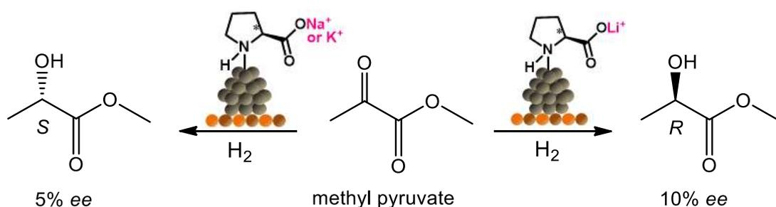
**Figure 8.** Hydrogenation of methyl pyruvate over PRO-functionalized Pt NPs coordinating different alkali metal cations.
