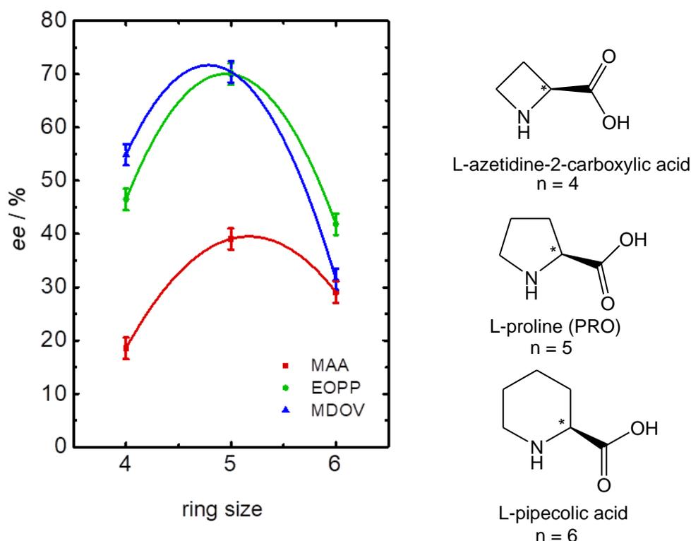
**Figure 5.** Effect of the ring size of the ligand on the stereoselectivity. Structures of the ligands are shown on the right. The solid lines are fits of the experimental data that serve merely as guides to the eye.
