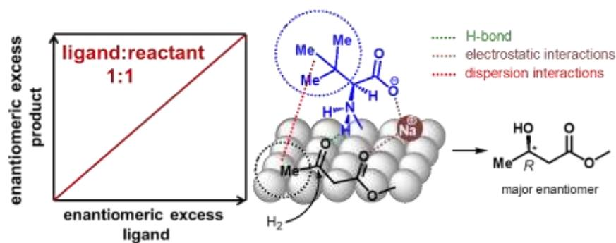
**Understanding of ligand-reactant interactions:** In the asymmetric hydrogenation of  $\beta$ -keto esters over  $\alpha$ -amino acid-functionalized supported Pt nanoparticles the stereoselectivity is mainly determined by a 1:1 ligand-reactant interaction and further influenced by small geometric changes in the ligand structure as well as by the alkali metal cation coordinated to the ligand.
