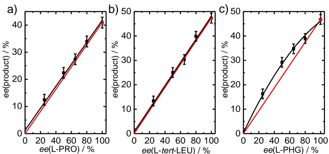
**Figure 2.** Relation between the product *ee* and the ligand *ee* for hydrogenation of MAA over Pt NPs functionalized with PRO (a), *tert*-LEU (b), and PHG (c). The solid lines are fits of the experimental data that serve merely as guides to the eye.
