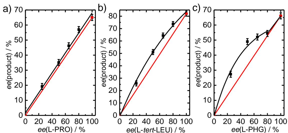
**Figure 3.** Relation between the product *ee* and the ligand *ee* for hydrogenation of MDOV over Pt NPs functionalized with PRO (a), *tert*-LEU (b), and PHG (c). The solid lines are fits of the experimental data that serve merely as guides to the eye.
