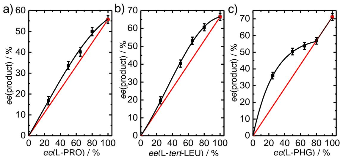
**Figure 4.** Relation between the product *ee* and the ligand *ee* for hydrogenation of EOPP over Pt NPs functionalized with PRO (a), *tert*-LEU (b), and PHG (c). The solid lines are fits of the experimental data that serve merely as guides to the eye.
