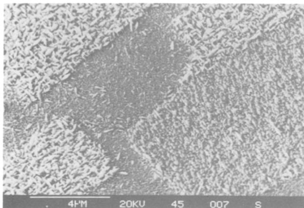
Fig. 3. A 500 nm thick dc-plated gold film deposited onto coarse-grained OFHC-Cu illustrating the difference in the transition substrate-controlled to bath-controlled growth compared with gold deposited onto fine-grained copper [Fig. 2(d)].
