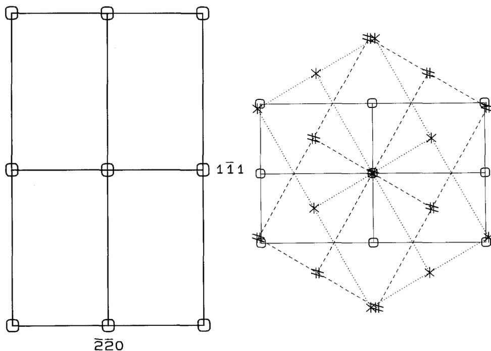
Fig. 6. In (a, left) a standard diffraction pattern from fcc,  $B = [112]$  is shown and, (b, right) illustrates three overlapping patterns identical with (a), mutually rotated  $120^\circ$  with respect to each other. This is how Fig. 4 (d) is built.
