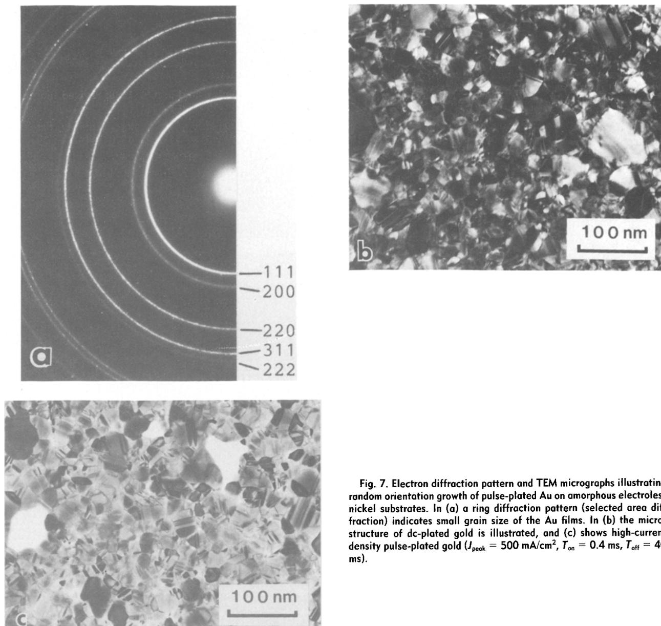
Fig. 7. Electron diffraction pattern and TEM micrographs illustrating random orientation growth of pulse-plated Au on amorphous electroless nickel substrates. In (a) a ring diffraction pattern (selected area diffraction) indicates small grain size of the Au films. In (b) the microstructure of dc-plated gold is illustrated, and (c) shows high-current density pulse-plated gold ( $J_{\text{peak}} = 500 \text{ mA/cm}^2$ ,  $T_{\text{on}} = 0.4 \text{ ms}$ ,  $T_{\text{off}} = 40 \text{ ms}$ ).
