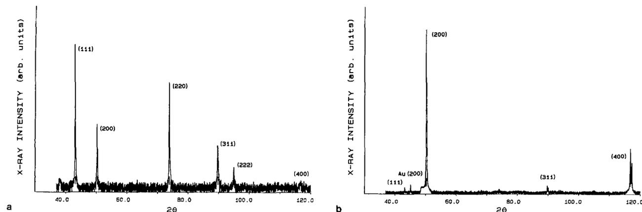
Fig. 4. X-ray diffractograms from Cu substrates. In (a) a diffractogram from electroformed Cu (Cu-epoxy) is shown. It exhibits a slightly increased intensity of the (220) reflection indicating a weak [110] texture. In (b) a diffractogram from OFHC-Cu is shown. The (200) reflection dominates completely indicating a strong [100] texture. The (400) and (311) reflections are also revealed.
