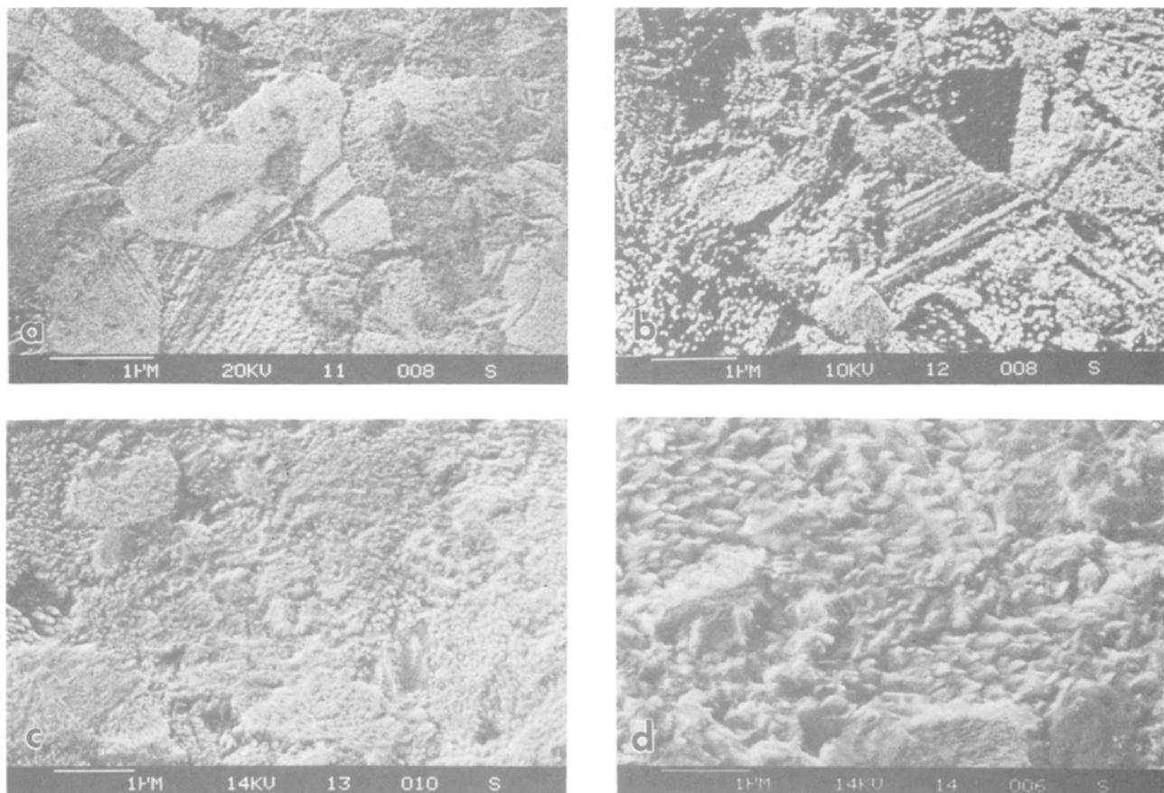
Fig. 1. Development of a gold film deposited under pulse plating conditions onto an electroformed copper substrate at gold thicknesses of (a) 10 nm, (b) 40 nm, (c) 150 nm, and (d) 500 nm.
