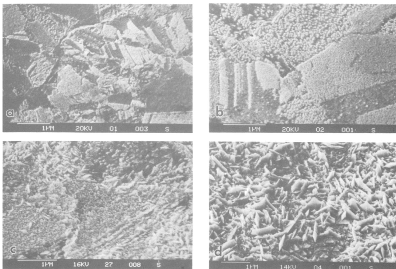
Fig. 2. Development of a gold film deposited under dc conditions onto an electroformed copper substrate at gold thicknesses of (a) 10 nm, (b) 50 nm, (c) 150 nm, and (d) 500 nm. A transition from epitaxial conditions to bath property–controlled conditions has started at a thickness of about 150 nm.
