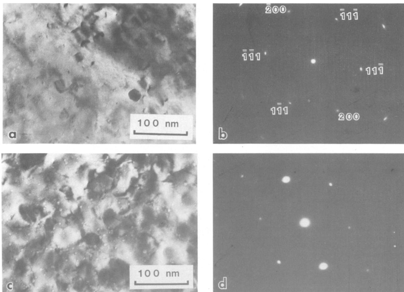
Fig. 5. TEM pictures and electron diffraction patterns showing the main growth orientations observed in 50 nm gold films. In (a) and (b) the single-crystalline structure of an epitaxial grain with [011] Au orientation is shown. In (c) and (d) a polycrystalline grain structure of [112] Au orientation is shown.
