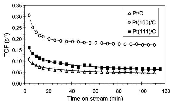
Fig. 4. TOF in crotonaldehyde hydrogenation at 333 K as a function of time on stream for Pt/C, Pt(111)/C, and Pt(100)/C catalysts.
