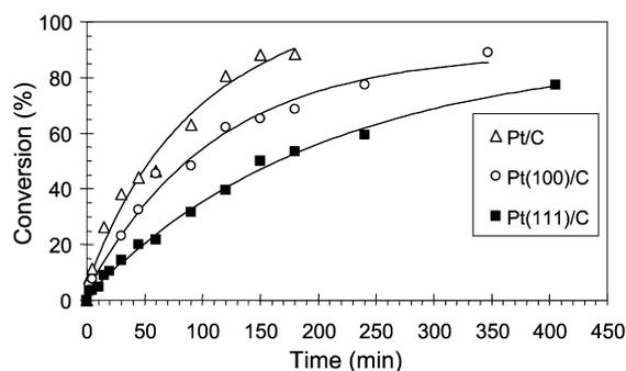
Fig. 6. Conversion of cinnamaldehyde as a function of time for Pt/C, Pt(111)/C, and Pt(100)/C catalysts.
