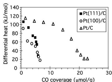
Fig. 3. Differential heats of CO adsorption at 300 K vs CO coverage for Pt/C, Pt(111)/C, and Pt(100)/C catalysts, previously reduced at 473 K.
