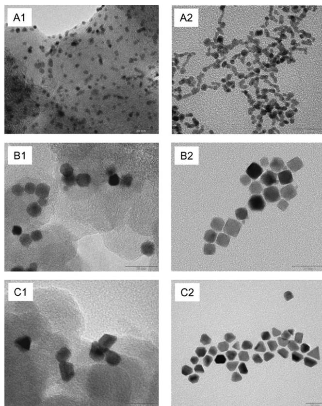
Fig. 1. TEM pictures corresponding to supported (1) and unsupported (2) Pt nanoparticles: polyoriented (A1, A2), preferentially oriented (100) (B1, B2), and preferentially oriented (111) (C1, C2) surface orientation.
