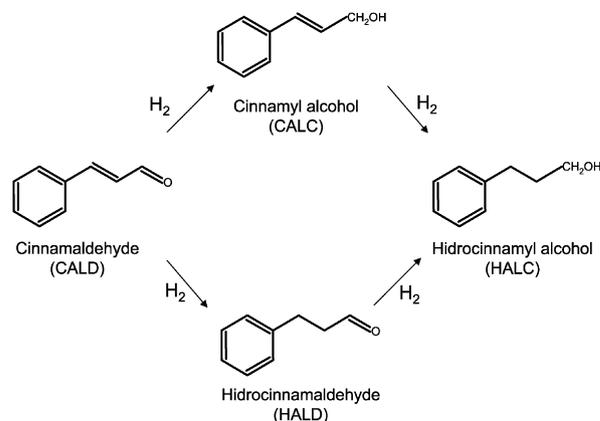
Fig. 5. Reaction scheme for cinnamaldehyde hydrogenation.
