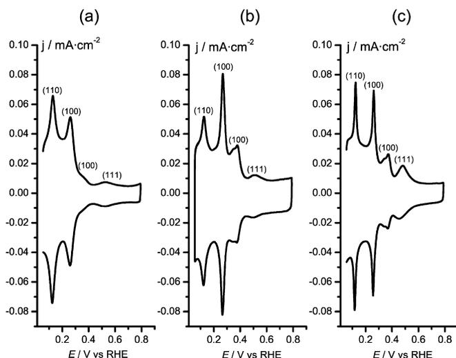
Fig. 2. Voltammograms corresponding to (a) poly, (b) (100), and (c) (111) Pt nanoparticles. Test solution: 0.5 M  $\text{H}_2\text{SO}_4$ , sweep rate  $50 \text{ mV s}^{-1}$ .
