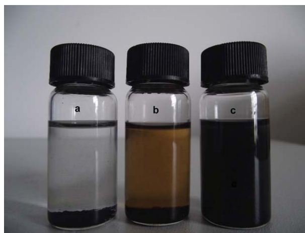
FIGURE 2 Comparison of solubility of the samples in THF: (a) MWNTs, (b) MWNT-COOH, and (c) MWNT-PCBF. The black dispersion shown in (c) is stable for at least 1 month. The concentration for each sample is 5 mg/mL.
