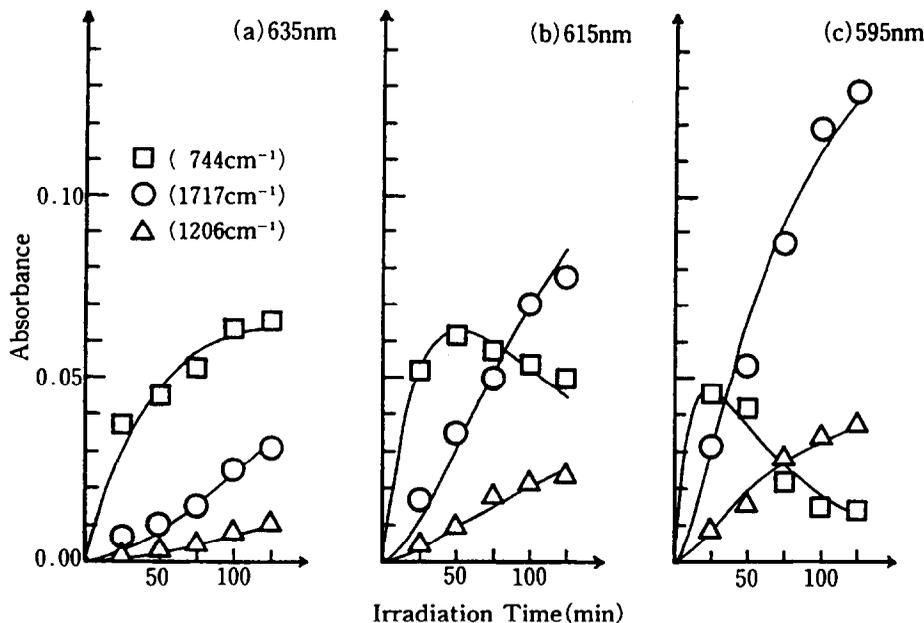
Fig. 6. Absorbance growth behaviour of IR bands of a photoreaction intermediate and two final products. Symbols  $\square$ ,  $\circ$  and  $\triangle$  denote the bands at 744 (nitrite radical), 1717 (K; 3,3-dimethyl-2-butanone) and  $1206\text{ cm}^{-1}$  (O; tetramethyloxirane). Wavelength of laser light is 635 (a), 615 (b) and 595 nm (c). Solid lines represent the calculated values using the rate constants listed in Table 4.
