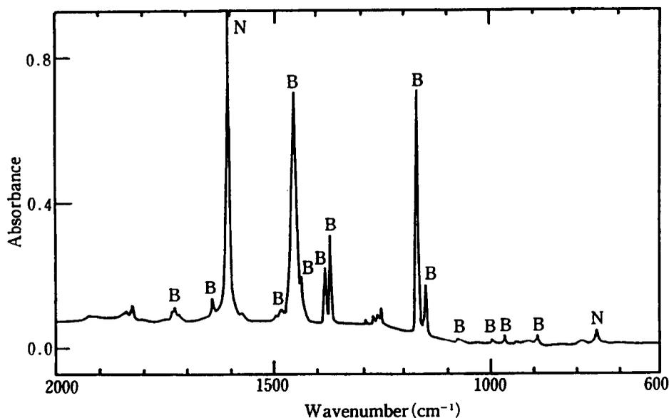
Fig. 2. IR spectrum of a "regular" matrix sample (2,3-dimethyl-2-butene-NO<sub>2</sub>-Ar, 2.5:1:100) before irradiation. The symbols N and B denote bands due to NO<sub>2</sub> and 2,3-dimethyl-2-butene, respectively. Other small bands are due to N<sub>2</sub>O<sub>3</sub> or N<sub>2</sub>O<sub>4</sub>.
