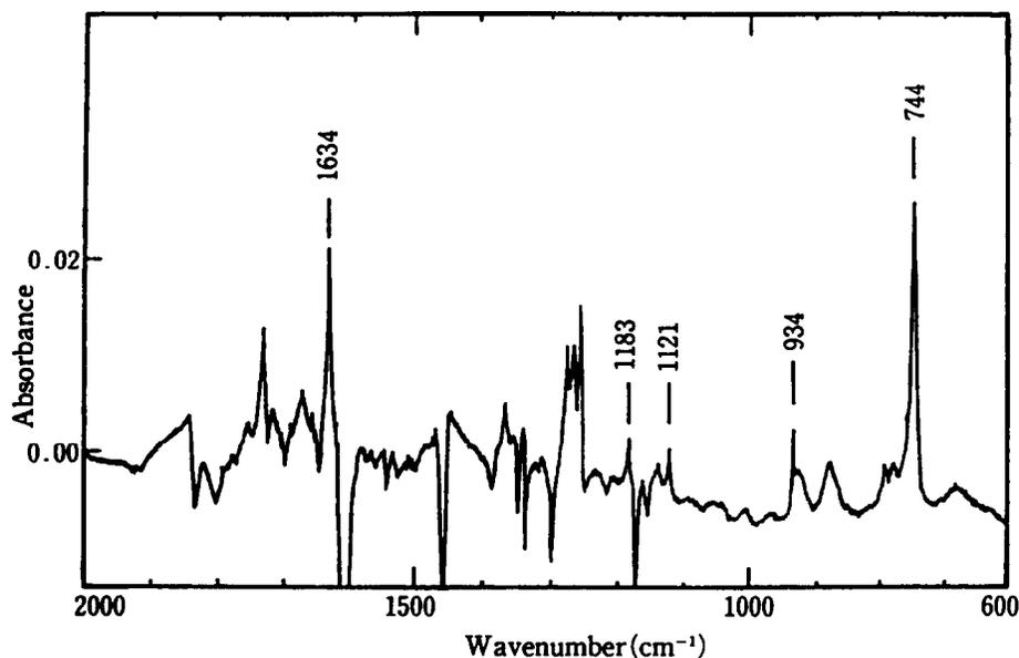
Fig. 3. Spectral change of a "dilute" matrix sample (2,3-dimethyl-2-butene-NO<sub>2</sub>-Ar, 2.5:1:400) upon 635 nm laser irradiation for 25 min. Five bands at 1634, 1183, 1121, 934 and 744 cm<sup>-1</sup> are due to an intermediate. Other spectral changes originate from N<sub>2</sub>O<sub>5</sub> isomerization.
