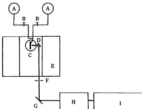
Fig. 1. Diagram of the experimental set-up. (A) Bulbs containing  $\text{NO}_2$ -Ar and 2,3-dimethyl-2-butene-Ar gas mixtures. (B) Needle valves. (C) Caesium iodide cold plate held at 20 K in a vacuum chamber. (D) Prism. (E) FTIR spectrophotometer, JASCO-8000S. (F) Aperture. (G) Mirror. (H) Dye laser, Spectra Physics Model 375B. (I) Argon ion laser, Spectra Physics Model 2016.
