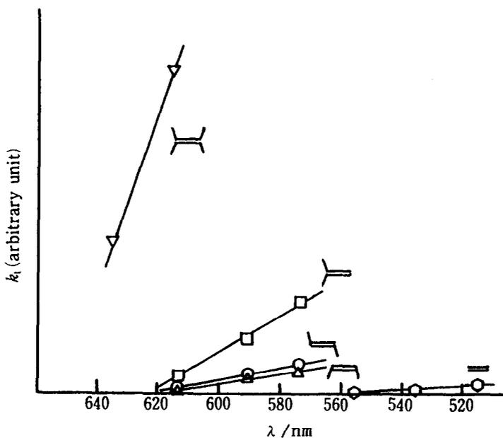
Fig. 7. A comparison of normalized rate constants,  $k_1+k_3$ , of photoreactions of  $\text{NO}_2$  with alkenes. Symbols  $\circ$ ,  $\Delta$ ,  $\square$  and  $\nabla$  represent ethylene, *cis*-2-butene, *trans*-2-butene, methylpropene and 2,3-dimethyl-2-butene, respectively. The obtained rate constants were normalized with respect to the laser photon density calculated from laser wavelength and laser power.
