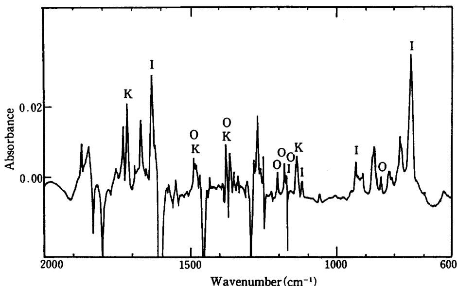
Fig. 5. Spectral change of a "regular" matrix sample (2,3-dimethyl-2-butene-NO<sub>2</sub>-Ar, 2.5:1:100) upon 635 nm laser irradiation for 25 min. Increasing bands are due to an intermediate (I, nitrite radical), and final products labelled K (3,3-dimethyl-2-butanone) or O (tetramethyloxirane).
