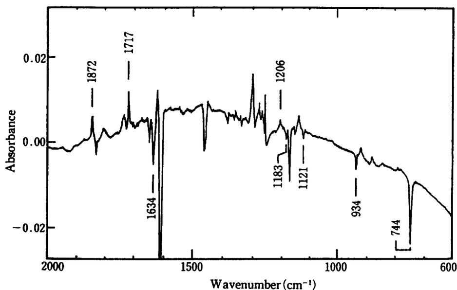
Fig. 4. Spectral changes of a "dilute" matrix sample (2,3-dimethyl-2-butene-NO<sub>2</sub>-Ar, 2.5:1:400) upon 570 nm laser irradiation for 10 min after accumulation of intermediate by 635 nm laser photolysis for 50 min. Decreasing bands are due to depletion of intermediate. Increasing bands are due to the final products NO (1872 cm<sup>-1</sup>), 3,3-dimethyl-2-butanone (1717 cm<sup>-1</sup>) and tetramethyloxirane (1206 cm<sup>-1</sup>).
