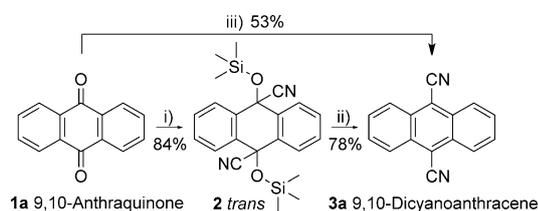
**Scheme 1.** Individually screened reaction steps from quinones to cyanoarenes by using 9,10-anthraquinone **1a** as the starting material: cyanohydrin formation (i) (Table 1), reductive aromatization (ii) (Table 2); synthesis finally carried out as a one-pot reaction (iii) (Table 3).
