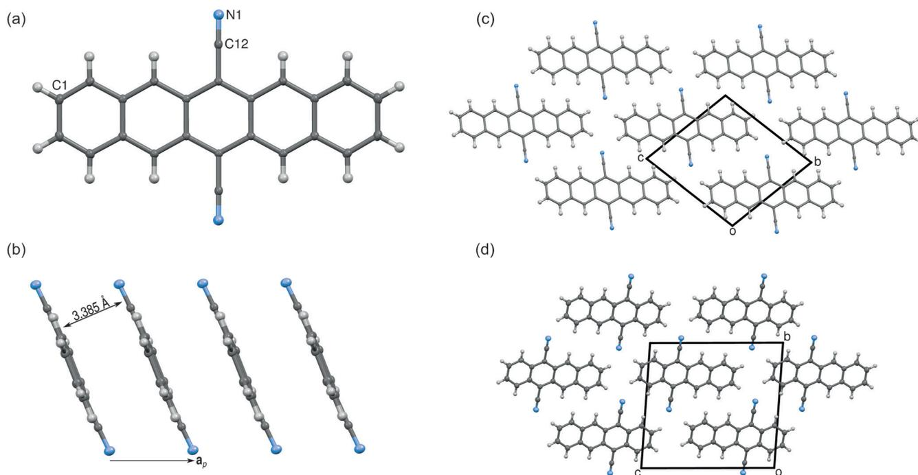
**Figure 3.** a) Molecular structure, b) rods of  $\pi$ -stacked molecules, and c) packing of 6,13-dicyanopentacene **15** viewed down [100]. d) Packing of 5,12-dicyanonaphthacene viewed down [100] (coordinates taken from Katsuta et al.<sup>[3]</sup>). Atom designations as in Figure 1.
