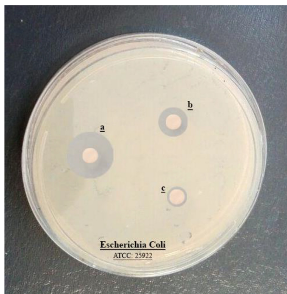
Fig. 10. Disk diffusion used to determine the antibacterial efficiency of Pd NPs@CS-Kao on E. coli .
