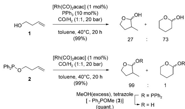
**Scheme 1.** Hydroformylation of homoallylic alcohol **1** with and without a covalently bound catalyst-directing phosphinite group (**2**). acac = acetylacetonate.
