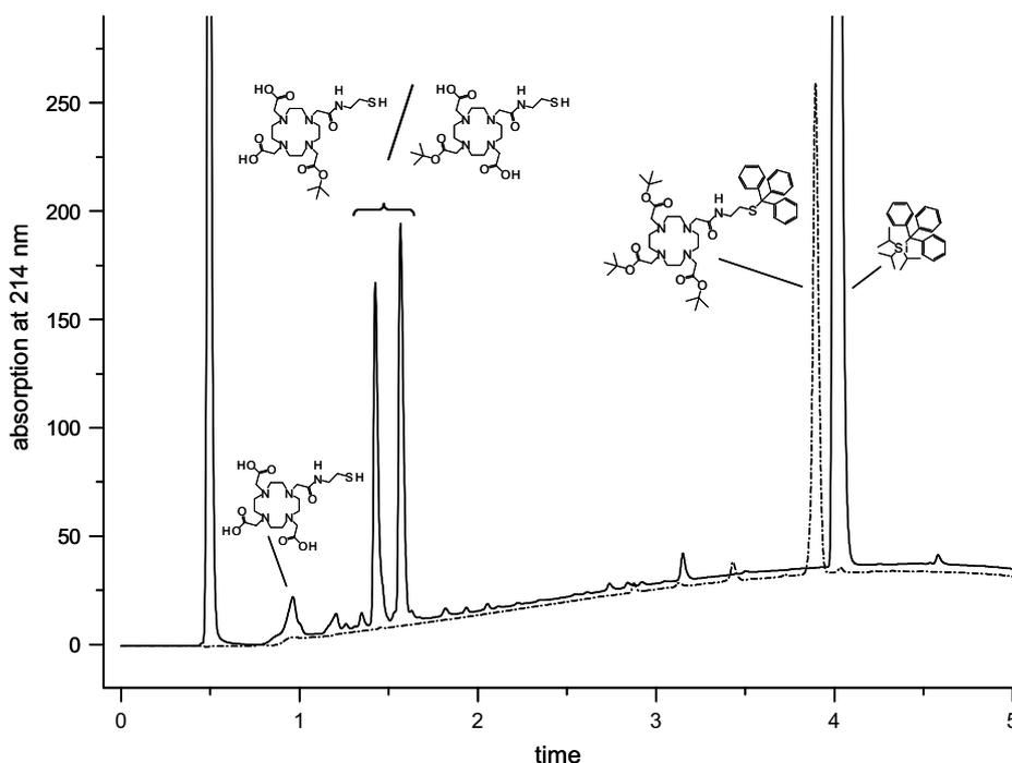
**Figure 1.** Chromatograms of the deprotection reaction of *S*-trityl-mercapto-*tris-t*Bu-DOTA with concentrated TFA after 16 h (compact line) and the educt (dashed line). Elution gradient: 0–100% MeCN + 0.1% TFA in 5 min.
