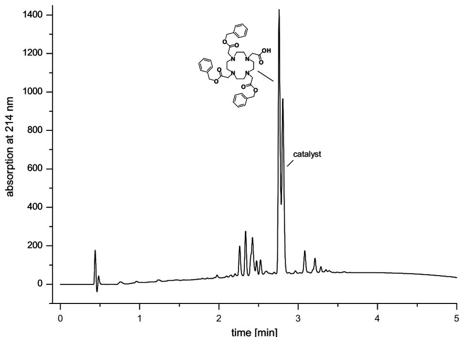
**Figure 4.** Chromatogram of the final deprotection step of **7** to tris-benzyl-DOTA with tetrakis-(triphenylphosphine)-palladium as catalyst after 3 h. Elution gradient: 0–100% MeCN + 0.1% TFA in 5 min.
