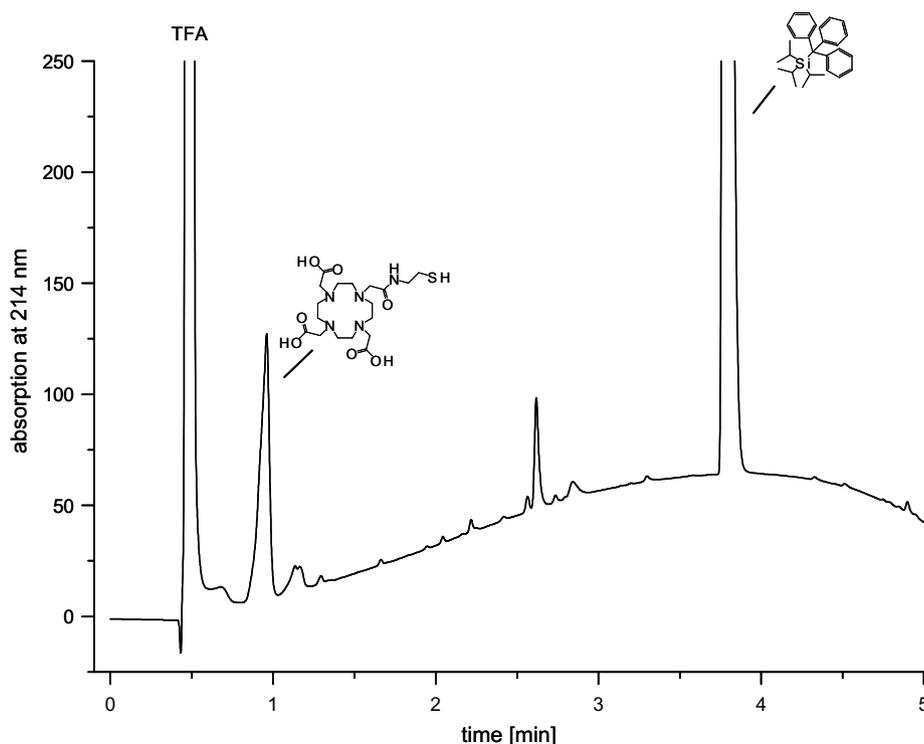
**Figure 2.** Chromatogram of the deprotection reaction of *S*-trityl-mercaptoethylamino-DOTA with concentrated TFA after 5 min. Elution gradient: 0–100% MeCN + 0.1% TFA in 5 min (note that the product does not contain a strong chromophore absorbing at 214 nm).
