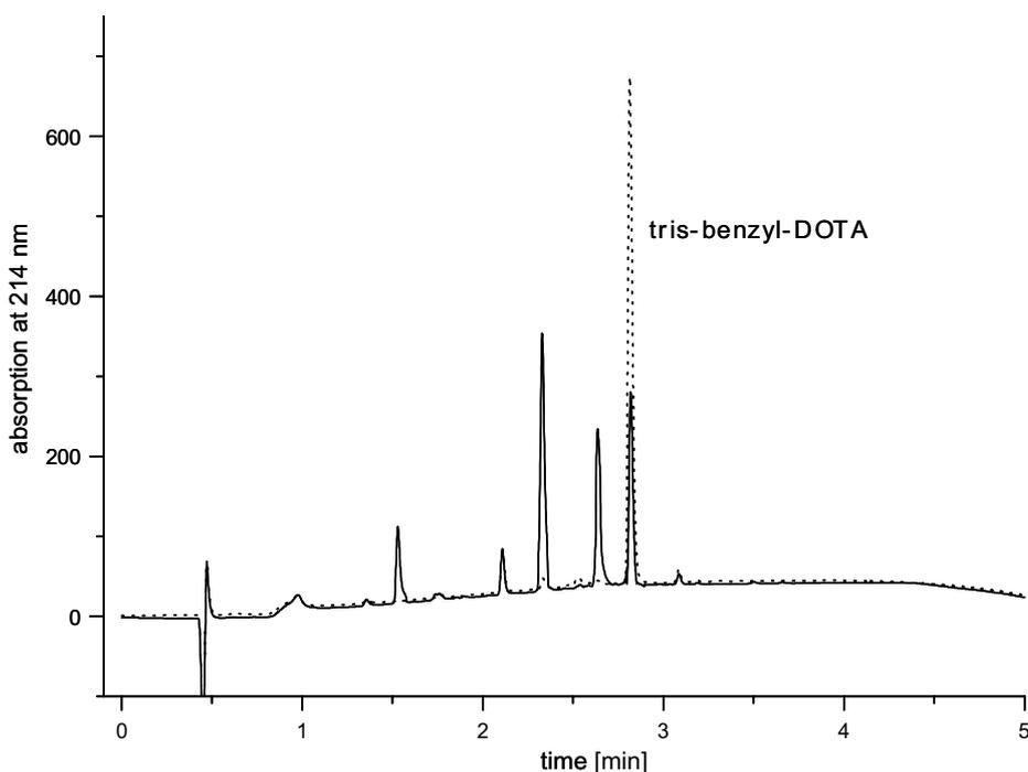
**Figure 3.** Decomposition of tris-benzyl-DOTA with 12 N HCl/dioxane 1:1 after 10 min (dashed line) and 12 h (compact line). Elution gradient: 0–100% MeCN + 0.1% TFA in 5 min.
