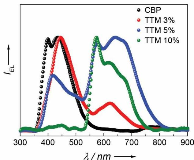
Figure 5. Electroluminescence of evaporated TTM OLED devices with different doping quantities.
