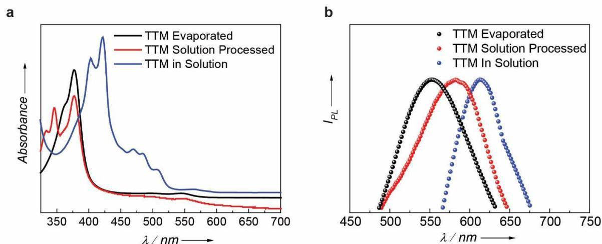
Figure 2. (a) UV-Visible absorption spectrum of evaporated TTM film, solution-processed TTM film and TTM in dichloromethane solution (b) The photoluminescence spectrum of TTM in dichloromethane solution and TTM evaporated as film.
