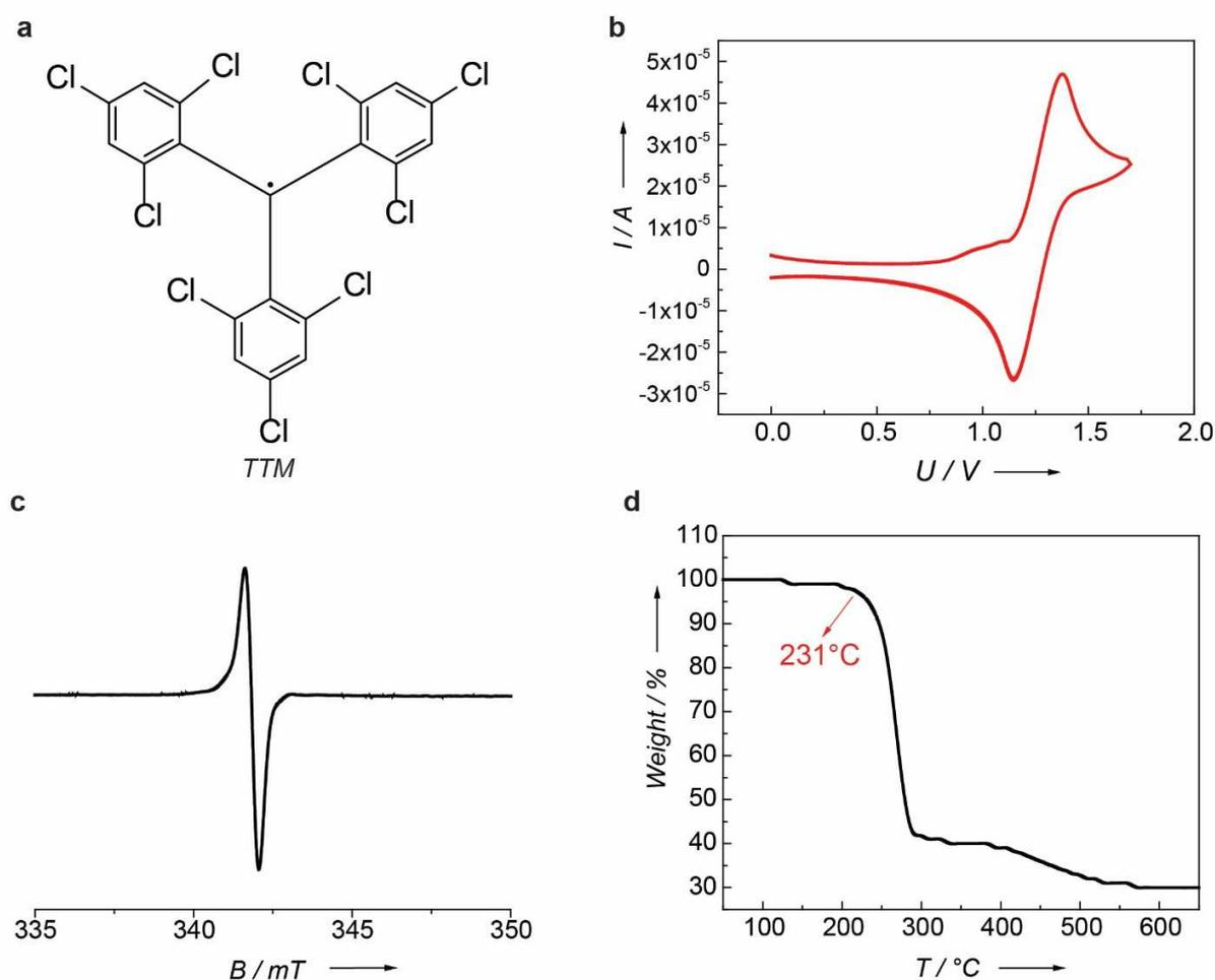
Figure 1. (a) Chemical structure of TTM (b) Cyclic-voltammetry in dichloromethane (c) The EPR spectrum in dichloromethane at room temperature (d) Thermogravimetric analysis spectrum of TTM
