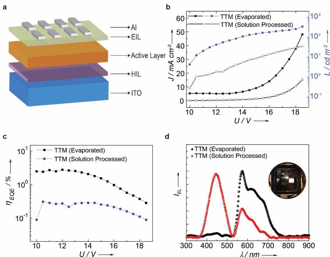
Figure 4 (a) Device structure of the TTM OLED. (b) J-V-L characteristics of the TTM OLED devices (c) External quantum efficiency of the OLED devices vs. voltage. (d) Electroluminescence of solution and evaporation based OLED devices. The inset shows an evaporated OLED device operating at 10 V.
