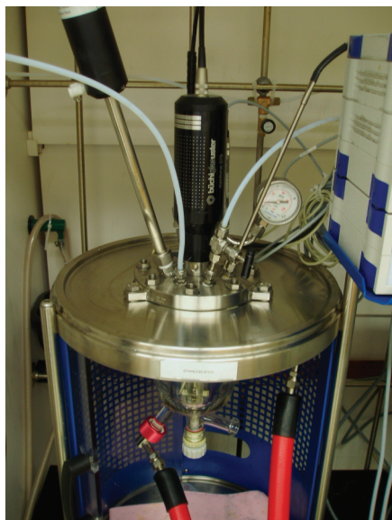
Figure 1. Introduction of the mid-IR probe into the hydrogenation vessel.
