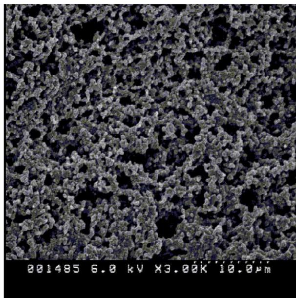
Figure 1. Cross-section of porous cross-linked material **10** (10  $\mu\text{m}$  per division on lower scale).
