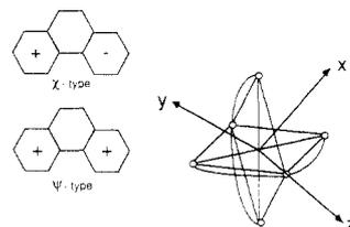
**Figure 8.** Symmetrized coordinate system chosen for a complex in  $D_{2d}$  symmetry with illustrations of the molecular orbital designations used for the ligands.
