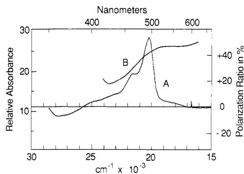
**Figure 2.** Absorption and polarization spectra of  $[\text{Cu}(\text{bcn})_2]\text{ClO}_4$  in 4:1 ethanol/methanol glass: A, absorption at 77 K; B, excitation polarization ratio at 100 K monitored at 750 nm.
