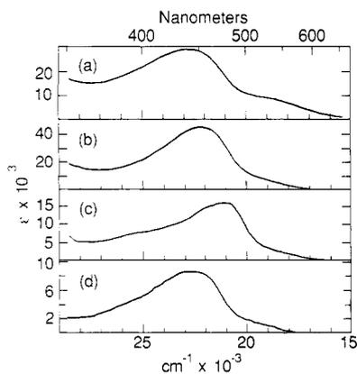
**Figure 1.** Effect of ligand modification on the visible absorption spectra of some cuprous complexes in 4:1 ethanol/methanol at room temperature: (a)  $[\text{Cu}(\text{bpy})_2]\text{ClO}_4$ ; (b)  $[\text{Cu}(\text{dmb})_2]\text{ClO}_4$ ; (c)  $[\text{Cu}(\text{bcn})_2]\text{ClO}_4$ ; (d)  $[\text{Cu}(\text{phen})_2]\text{ClO}_4$ .
