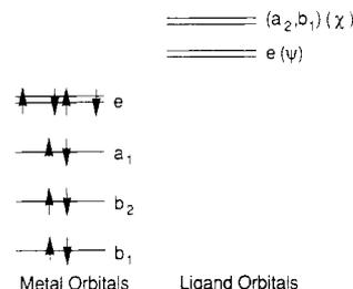
**Figure 7.** Proposed orbital scheme for  $[\text{Cu}(\text{NN})_2]^+$  ions in  $D_{2d}$  symmetry. The  $\Psi$  and  $\chi$  labels refer to individual ligand orbitals that are antisymmetric ( $\Psi$ ) and symmetric ( $\chi$ ) with respect to the principal  $C_2$  axis of the complex. These form the basis for the indicated representations in  $D_{2d}$ .
