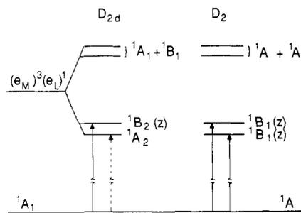
Figure 9. Proposed singlet energy level scheme for  $[\text{Cu}(\text{NN})_2]^+$  complexes:  $\rightarrow$  allowed transition;  $-\rightarrow$  forbidden transition.
