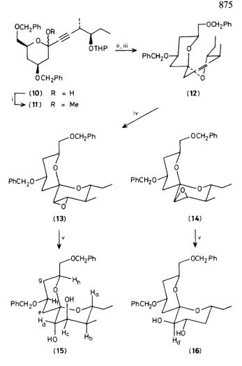
Reagents: i, MeOH-H<sup>+</sup>; ii, Lindlar catalyst-MeOH-H<sub>2</sub>; iii, CSA-CH<sub>2</sub>Cl<sub>2</sub>; iv, MCPBA; v, HClO<sub>4</sub>.
