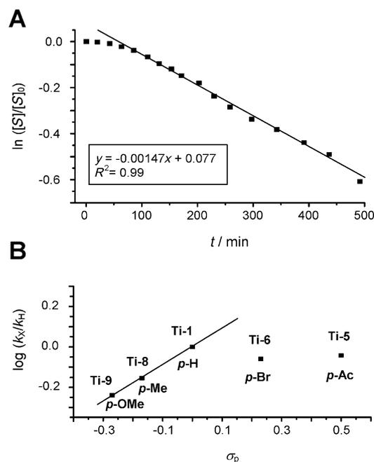
**Figure 5.** A) Kinetics of styrene epoxidation ( $\text{CH}_2\text{Cl}_2$ , 290 K) by catalyst system Ti-1/ $\text{H}_2\text{O}_2$  and its linear fit, with the exception of first four points. B) Hammett plot of  $\log(k_x/k_h)$  for styrene epoxidations with  $\text{H}_2\text{O}_2$  in the presence of various titanium catalysts, and its linear fit performed for catalysts Ti-9, Ti-8 and Ti-1.
