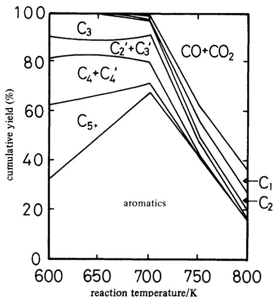
Fig. 3. Change in the product distribution with reaction temperature in methanol conversion over Zn-ZSM-5.  $P(\text{MeOH}) = 40 \text{ kPa}$ ,  $W/F = 9.0 \text{ g h mol}^{-1}$ .
