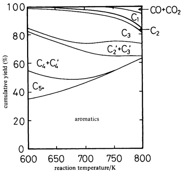
**Fig. 2.** Change in the product distribution with reaction temperature in methanol conversion over Ga-ZSM-5.  $P(\text{MeOH}) = 40 \text{ kPa}$ ,  $W/F = 9.0 \text{ g h mol}^{-1}$ .
