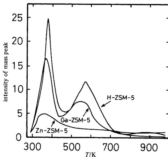
Fig. 9. Temperature-programmed desorption of ammonia from H-ZSM-5, Ga-ZSM-5 and Zn-ZSM-5.
