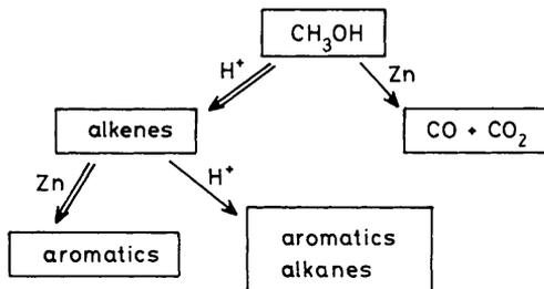
Fig. 10. Reaction scheme of methanol conversion over Zn-ZSM-5.
