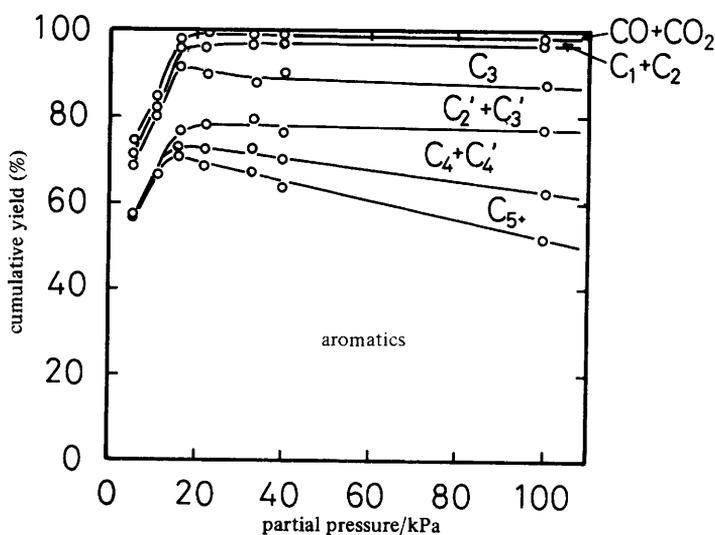
**Fig. 4.** Change in the product distribution with the methanol partial pressure for the methanol conversion over Zn-ZSM-5. *T* = 700 K, *W/F* = 9.0 g h mol<sup>-1</sup>.
