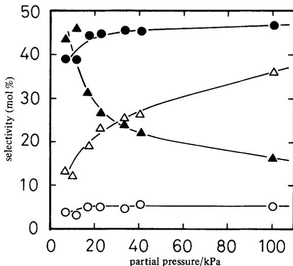
**Fig. 5.** Effect of the methanol partial pressure on the selectivity among aromatic hydrocarbons produced in the methanol conversion over Zn-ZSM-5.  $T = 700$  K,  $W/F = 9.0$  g h mol<sup>-1</sup>. ○, Benzene; △, toluene; ●, C<sub>8</sub>; ▲, C<sub>9+</sub>.
