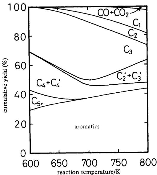
**Fig. 1.** Change in the product distribution with reaction temperature in methanol conversion over H-ZSM-5.  $P(\text{MeOH}) = 40 \text{ kPa}$ ,  $W/F = 9.0 \text{ g h mol}^{-1}$ .
