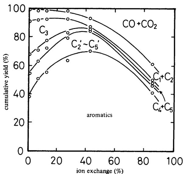
**Fig. 8.** Change in the product distribution with the degree of cation exchange of H-ZSM-5 with zinc cations for the methanol conversion.  $750$  K,  $P(\text{MeOH}) = 22$  kPa,  $W/F = 9.0$  g h mol<sup>-1</sup>.
