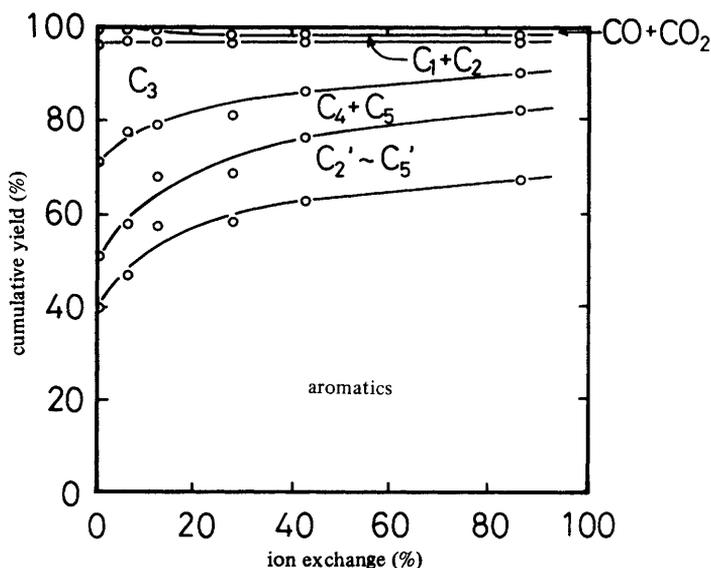
**Fig. 7.** Change in the product distribution with the degree of cation exchange of H-ZSM-5 with zinc cations for the methanol conversion.  $T = 700$  K,  $P(\text{MeOH}) = 22$  kPa,  $W/F = 9.0$  g h mol<sup>-1</sup>.
