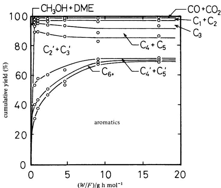
**Fig. 6.** Change in the product distribution with contact time for the methanol conversion over Zn-ZSM-5.  $T = 700$  K,  $P(\text{MeOH}) = 22$  kPa.
