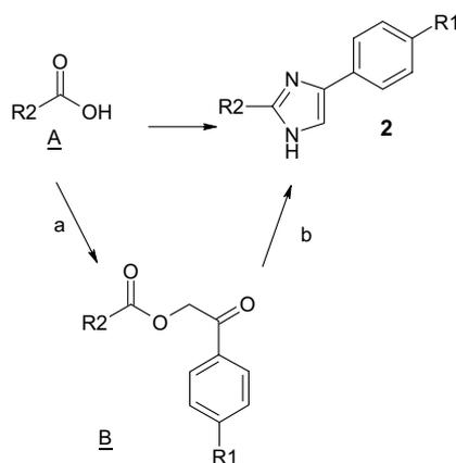
**Scheme 1.** One-pot formation of arylimidazoles **2**. (a) (i)  $\text{Cs}_2\text{CO}_3$ , MeOH, rt, (ii)  $\text{ArCOCH}_2\text{Br}$ , DMF, rt; (b)  $\text{NH}_4\text{OAc}$ , xylene, reflux with Dean-Stark.
