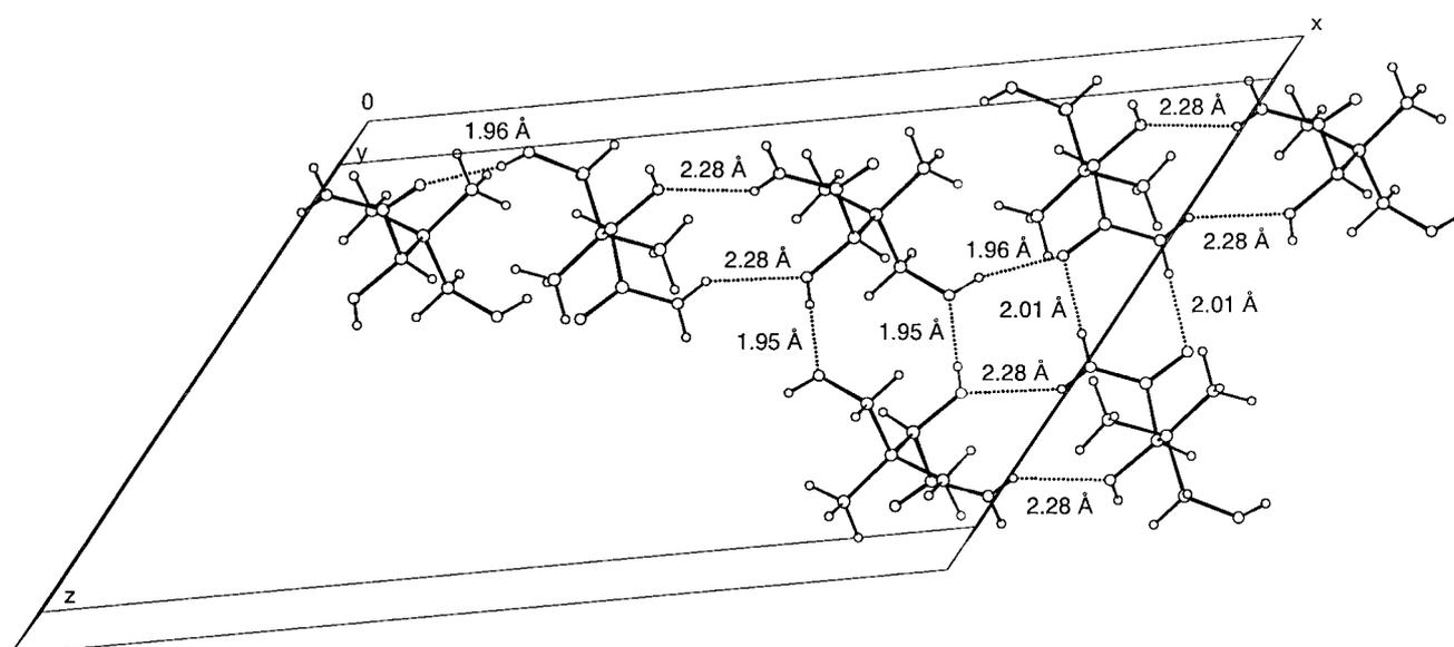
**Figure 6** Crystal packing of (*R,S*)-**2**, showing the presence of a hydrogen bond network.
