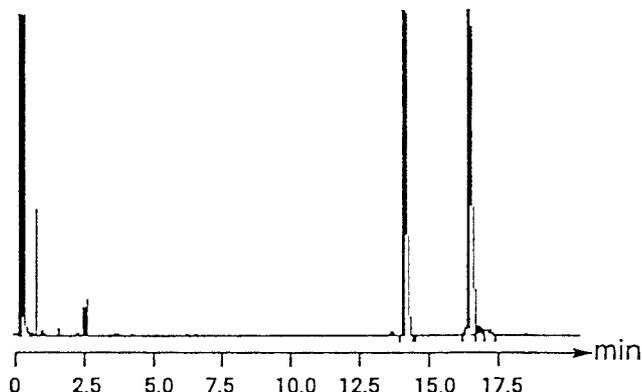
**Figure 1** Gas chromatogram of (*R,S*)-**5** (chiral stationary phase) after derivatization to the acetate. The GC conditions are described in the experimental part.
