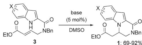
**Scheme 2.** Base-catalyzed synthesis of **1**. Bn: benzyl; DMSO: dimethylsulfoxide.
