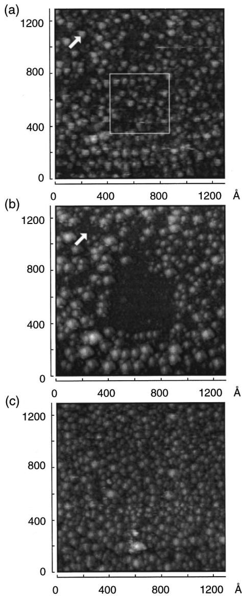
FIG. 1. (a) A region of passivated gold nanocrystals on graphite imaged at 30 pA and  $-1.5$  V sample bias. (b) The same region imaged at 30 pA ( $-1.5$  V) after twice scanning over the central region (indicated by white square) at 30 nA ( $-15$  V). This area has been cleared by the tip. (c) A densely packed cluster layer which was unchanged after the same scanning sequence as that used between (a) and (b).
