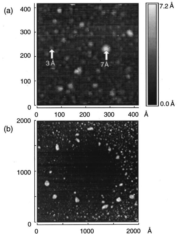
FIG. 2. (a) A region of cleared surface showing in cluster fragments: larger  $\sim 7$  Å high and smaller  $\sim 3$  Å high fragments are indicated. This image was acquired with tunneling current 5.8 nA and 1.5 V sample bias. (b) Repeated high current imaging causes displacement of the fragments. A circle of large faceted islands is shown. A sample bias of 1.5 V and tunneling current of 30 pA were used for this image.
