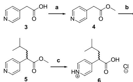
**Scheme 3.** Synthesis of 4-methyl-2-(pyridin-4-yl)pentanoic acid (**6**). Reagents and conditions: (a) i—MeOH, cat. H<sub>2</sub>SO<sub>4</sub>, reflux; ii—NaOH, H<sub>2</sub>O (quant.); (b) i—NaH, DMF, 0 °C; ii—1-bromo-2-methylpropane, 50 °C (68%); (c) 6 M HCl (quant.).
