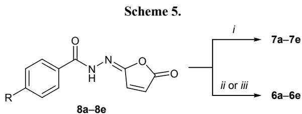
*i*: PhMe, reflux, 1.5 h; *ii*: AcOH, reflux, 4 h; *iii*: AcCl, CH<sub>2</sub>Cl<sub>2</sub>, 24 h, 20°C.
