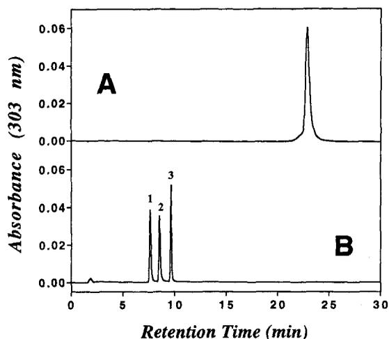
FIGURE 3. Reversed-phase HPLC characterization of the 16mer methylphosphonate containing exclusive 2-aminopurine base (**9**). Column: Microsorb C18 4.6x250mm. Detection: A303nm. Elution: linear 2-30% ACN gradient in 50 mM sodium phosphate, pH 7. (A): HPLC purified **9**. (B): piperidine-digested **9**, peak 1 and 2: 2-aminopurine-2'-deoxyribose-3' (or 5')-methylphosphonic acid, peak 3: 2-aminopurine-2'-deoxyribose.
