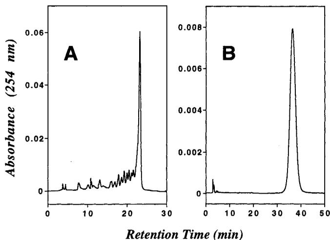
FIGURE 1. Polar stationary phase HPLC analysis of a 16mer methylphosphonate oligomer containing alternating 2-aminopurine and guanine bases (**8**). Column: Cyclobond 250 x 4.6mm. Detection: A254nm. (A): Crude **8**, linear 80% to 20% ACN gradient in 25 mM NH<sub>4</sub>OAc over 30min. (B): HPLC purified **8**, isocratic 55% ACN in 25mM NH<sub>4</sub>OAc.
