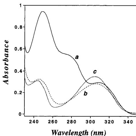
FIGURE 2. UV spectra of oligodeoxyribonucleoside methylphosphonates containing 2-aminopurine residues. (a): alternating 2-aminopurine-guanine 16mer **8** (6.25  $\mu$ M strand). (b): 2-aminopurine 16mer **9** (3.125  $\mu$ M strand). (c) 2-aminopurine-2'-deoxyribose (50  $\mu$ M). Solvent: 10% ACN in 10 mM sodium phosphate, pH 7.
