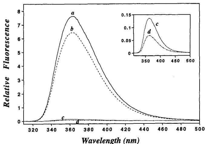
FIGURE 4. Fluorescence emission spectra of 2-aminopurine nucleosides and methylphosphonate oligomers. Each sample contains 5  $\mu$ M 2-aminopurine residues. Solvent: 10% ACN in 10 mM sodium phosphate, pH 7. Excitation wavelength: 303nm. (a): piperidine digested **9**. (b): 2-aminopurine-2'-deoxyribose. (c): alternating 2-amino-purine-guanine 16mer **8**. (d): 2-aminopurine 16mer **9**.
