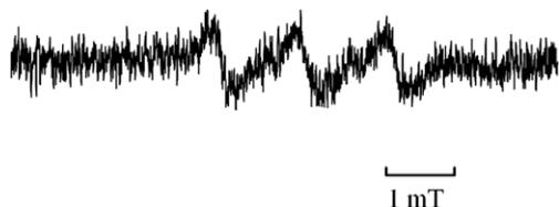
**Figure 4.** ESR spectra of [(DET)<sub>2</sub>-Fe-NO] complex after 840 nm pulse laser irradiation in the presence of **TB2-DNB**. Samples contained 250 μM **TB2-DNB**, 8 mM DETC, and 2 mM FeSO<sub>4</sub> in DMSO; ESR spectra were recorded after photoirradiation for 8 min with a modulation width of 0.5 G and a microwave power of 10 mW.
