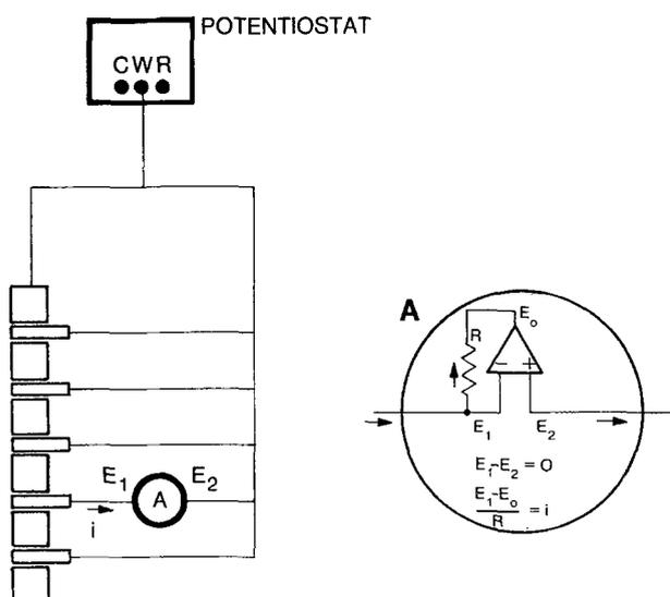
Fig. 3. Circuit for maintaining equal potential on probe
