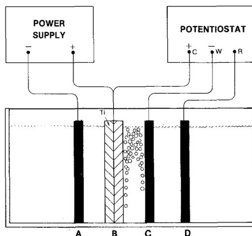
Fig. 2. Experimental setup for limiting current measurements. A, Auxiliary electrode: dense graphite. B, Gas-evolving electrode: titanium-sprayed porous graphite. C, Working electrode: dense graphite. D, Reference electrode: porous graphite,  $\text{Cl}_2/\text{Cl}^-$ .
