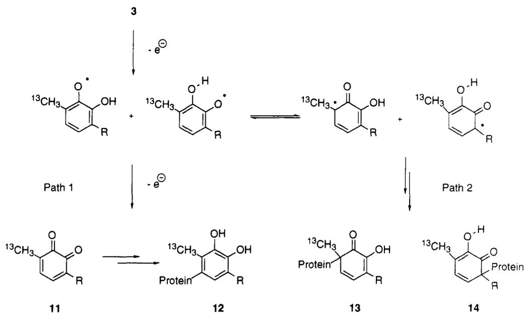
Scheme 2: Possible reaction pathways of **3** with HSA in phosphate buffer at pH 7.4 in the presence of oxygen
