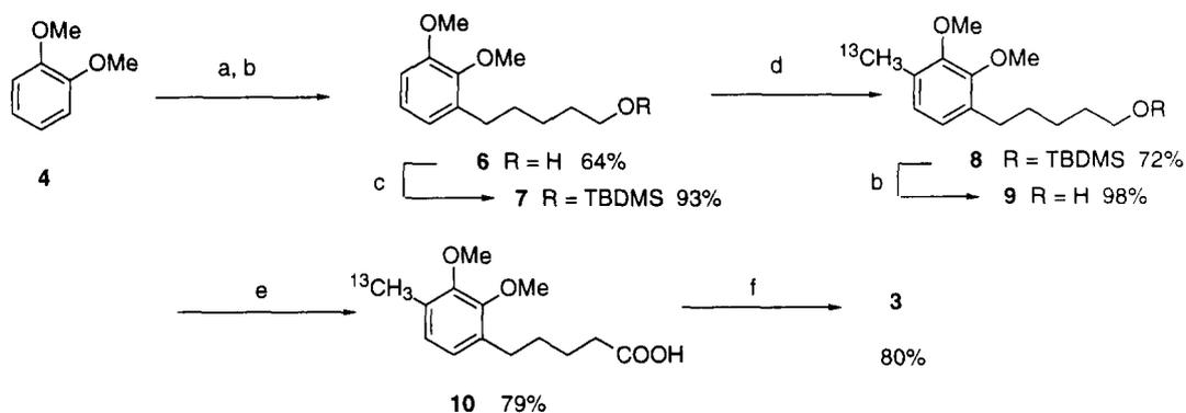
**Scheme 1:** (a) *n*-BuLi, THF then I-(CH<sub>2</sub>)<sub>5</sub>-OTBDMS; (b) TBAF, THF; (c) TBDMSCl, imidazole, DMF; (d) *s*-BuLi, TMEDA, Et<sub>2</sub>O then [<sup>13</sup>C]MeI; (e) PDC, DMF; (f) BBr<sub>3</sub>, CH<sub>2</sub>Cl<sub>2</sub>, -78°C.
