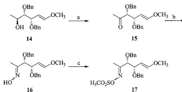
Scheme 5. Reagents and conditions: a) PDC, CH<sub>3</sub>CN, 4-Å molecular sieves, room temp. (95%); b) NH<sub>2</sub>OH·HCl, NEt<sub>3</sub>, EtOH/THF 1:1, 40 °C (80%); c) CH<sub>3</sub>SO<sub>2</sub>Cl, NEt<sub>3</sub>, CH<sub>2</sub>Cl<sub>2</sub>, room temp. (90%)
