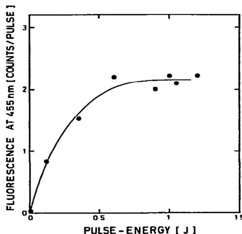
Fig. 2 Dependence of the fluorescence enhancement observed at 455 nm ( $22000\text{ cm}^{-1}$ ) on  $\text{CO}_2$ -laser pulse energy. Visible excitation wavelength 532 nm,  $\text{CO}_2$ -laser line  $949.5\text{ cm}^{-1}$
