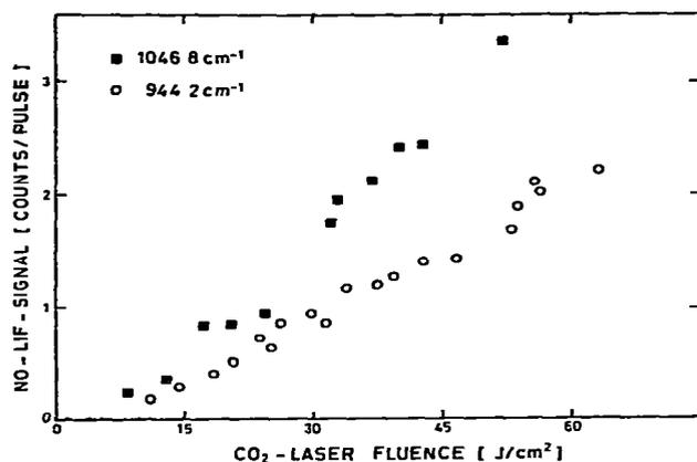
Fig. 6 CO<sub>2</sub>-laser fluence dependence of the NO dissociation yield, measured as under fig. 4. Visible excitation at 532 nm (18797 cm<sup>-1</sup>), CO<sub>2</sub>-laser lines at 1046.8 cm<sup>-1</sup> and 944.2 cm<sup>-1</sup>.
