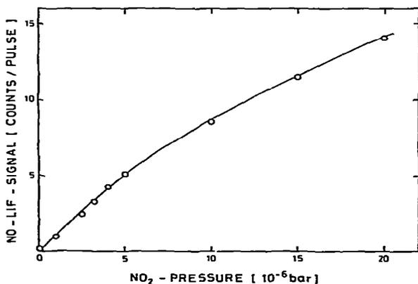
Fig. 4. NO<sub>2</sub> pressure dependence of the NO dissociation yield, measured by the LIF intensity of NO excited in the P<sub>11</sub> band head. Visible excitation at 435.7 nm, CO<sub>2</sub>-laser line 1046.8 cm<sup>-1</sup>.
