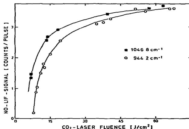
Fig. 5. CO<sub>2</sub>-laser fluence dependence of the NO dissociation yield measured as under fig. 4. Visible excitation at 435.7 nm (22952 cm<sup>-1</sup>), CO<sub>2</sub>-laser lines at 1046.8 cm<sup>-1</sup> and 944.2 cm<sup>-1</sup>.
