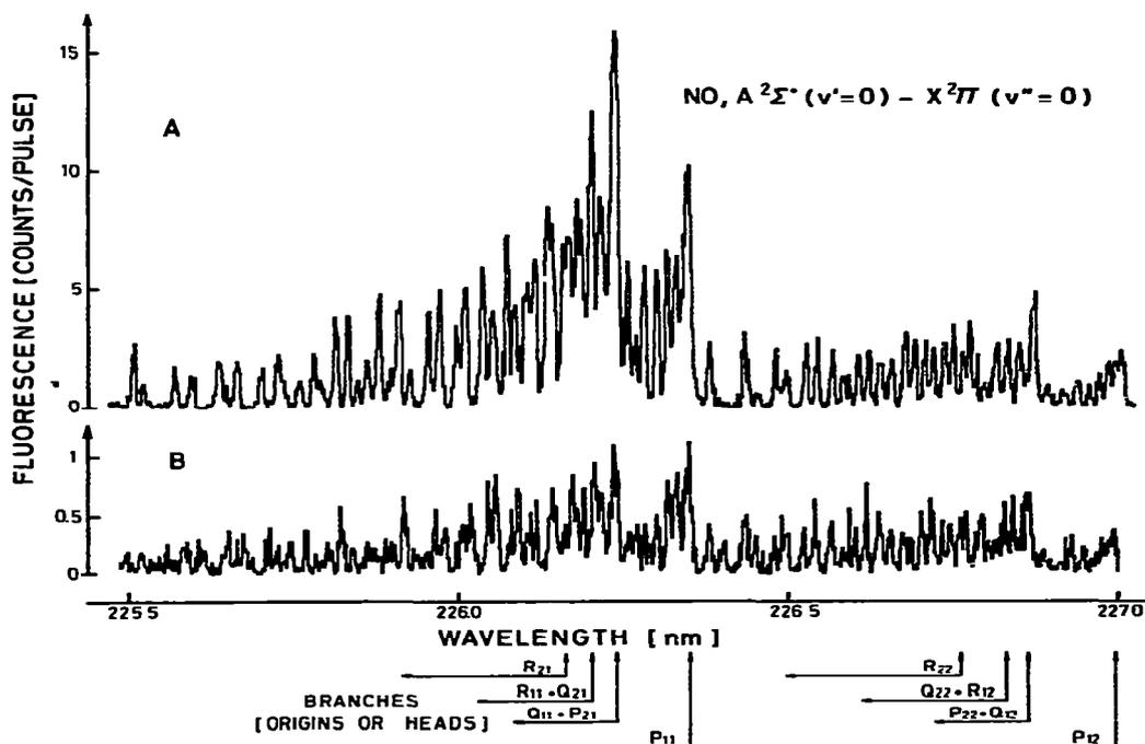
Fig. 3.  $\text{NO}_2$  dissociation by (1 VIS +  $n$  IR)-photon absorption. Excitation spectra of NO ( $A^2\Sigma^+, v' = 0 \leftarrow X^2\Pi, v'' = 0$ ). Upper spectrum (A).  $\text{NO}_2$  irradiated by 435.7 nm (energy 1 mJ/pulse) plus  $\text{CO}_2$ -laser light at  $944.2\text{ cm}^{-1}$  (energy 1 J/pulse),  $\text{NO}_2$  pressure  $3 \times 10^{-6}$  bar. Lower spectrum (B) NO background excitation spectrum. Conditions as in (A), however without  $\text{CO}_2$ -laser irradiation.
