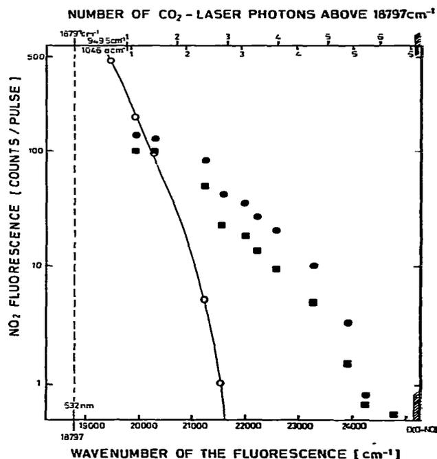
Fig. 1. Fluorescence of  $\text{NO}_2$  excited by (1 VIS +  $n$  IR)-photon absorption. Spectral fluorescence distribution produced by 532 nm alone (open circles); fluorescence enhancement by  $\text{CO}_2$ -laser radiation of  $1046.8 \text{ cm}^{-1}$  (full squares) and  $949.5 \text{ cm}^{-1}$  (full circles).  $\text{CO}_2$ -laser energy: 1 J/pulse.  $\text{NO}_2$  pressure:  $5 \times 10^{-6}$  bar at signals smaller than 10 counts/pulse,  $0.5 \times 10^{-6}$  bar at higher signals.
