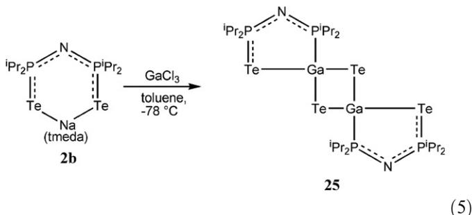
In an attempt to elucidate the pathway involved in the formation of the  $\text{Ga}_2\text{Te}_2$  ring, the reaction of **2b** with  $\text{GaCl}_3$
