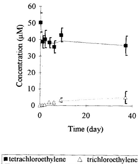
Figure 2. PCE dechlorination by the mixed culture supplemented with 10 mM BESA (Mean  $\pm$ SD).
