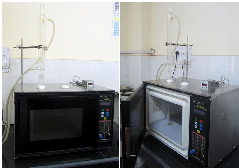
**Fig. 1** Catalyst system scientific microwave
