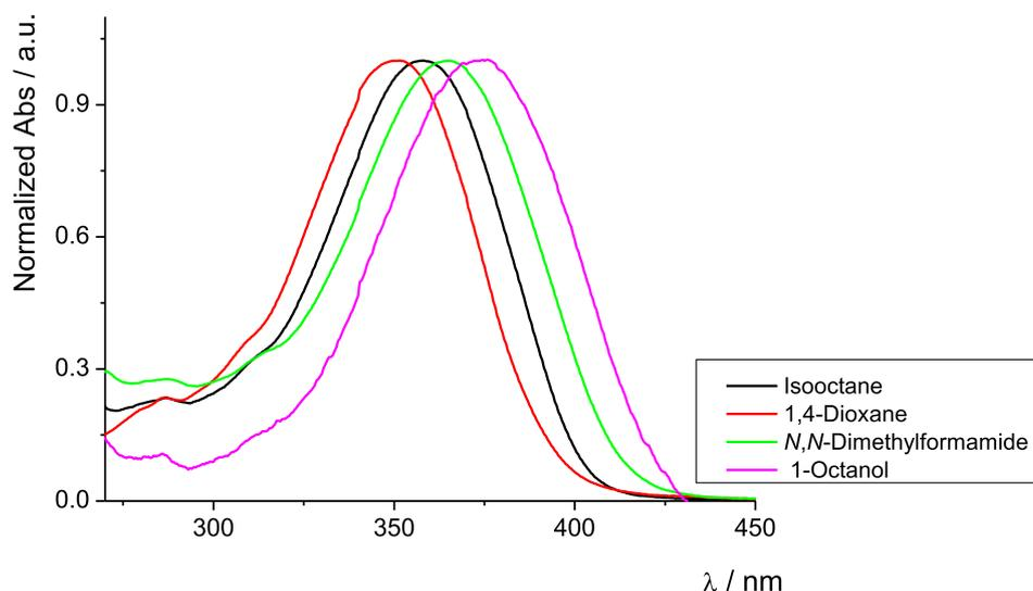
Fig. 5. Normalized UV-vis spectra of CyCUR in different solvents at 298 K.
