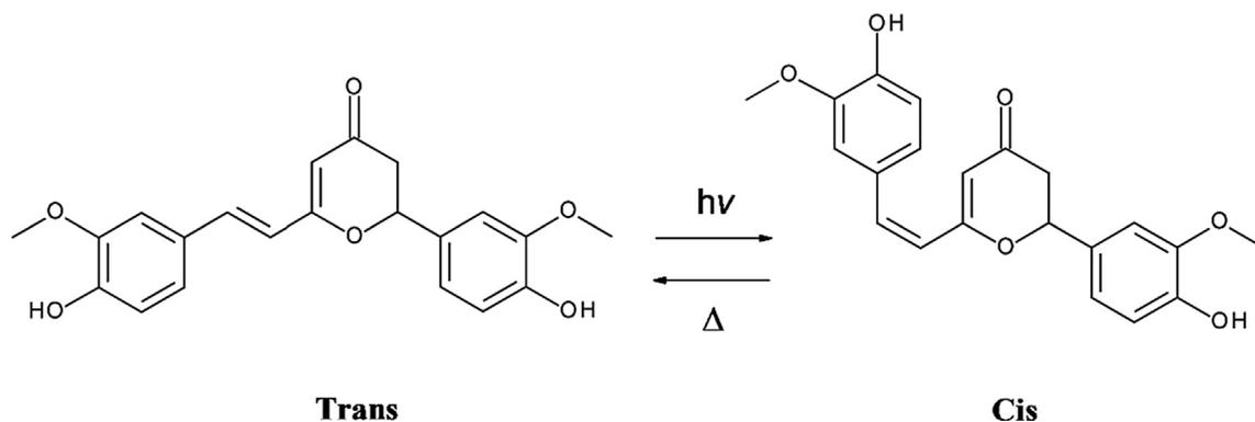
**Scheme 1.** Representation of the trans-cis and cis-trans isomerization of cyclocurcumin.
