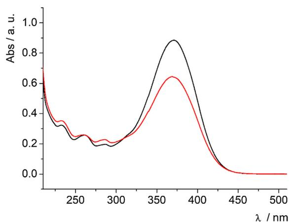
Fig. 1. UV–vis spectra of  $3 \times 10^{-5}$  M CyCUR in ethanol before (black line) and after irradiation (red line) at 365 nm.
