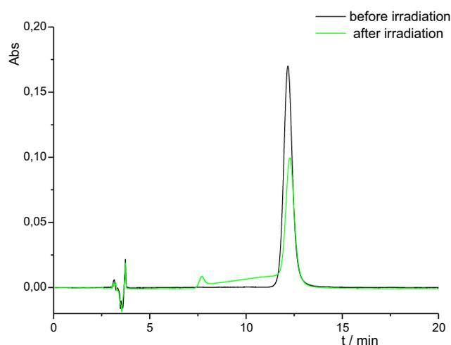
Fig. 2. Chromatograms of CyCUR in ethanol injected before (black line) and after irradiation (green line) at 365 nm.
