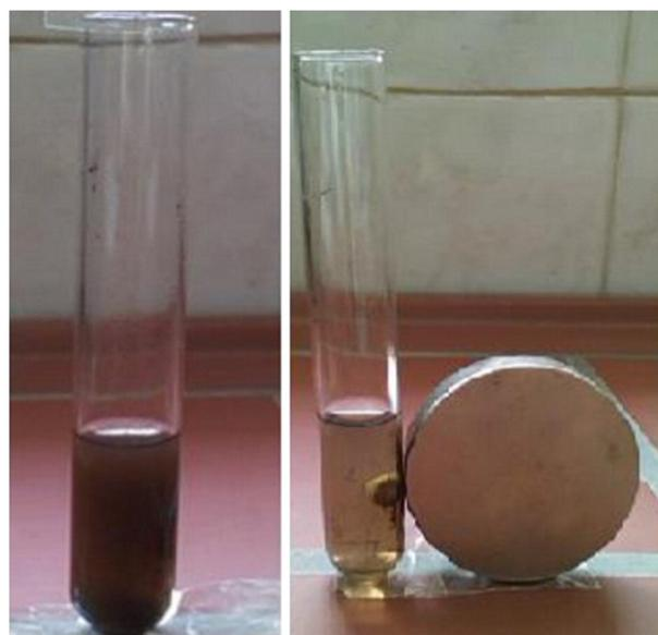
**Fig. 3.** A reaction mixture in the absence (left) or presence of a magnetic field (right).
