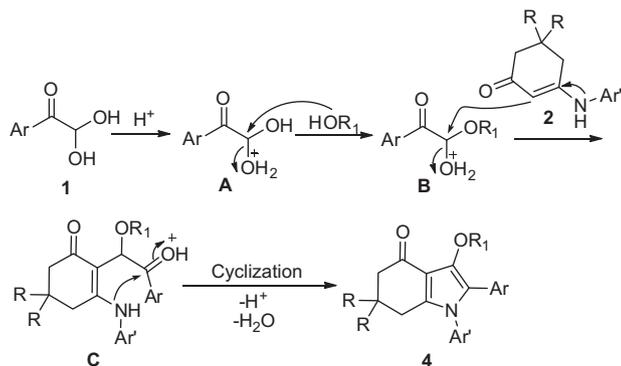
Scheme 2. The possible mechanism for tetrahydroindoles **4**.
