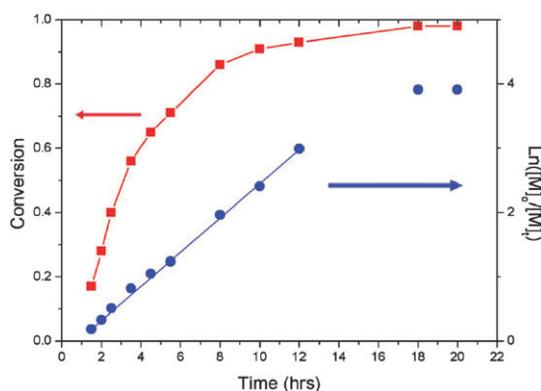
**Fig. 1** Conversion as a function of polymerisation time and pseudo-first-order kinetic plot for polymerisation of MMA via macro-RAFT agent in scCO<sub>2</sub>.
