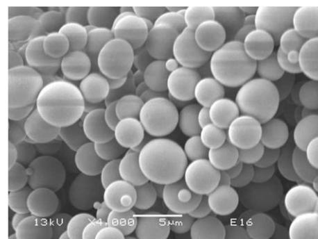
**Fig. 3** SEM image of PMMA particles formed by dispersion polymerisation in scCO<sub>2</sub> using macro-RAFT agent demonstrating well-defined, discrete particles of controlled molecular weight block copolymer.
