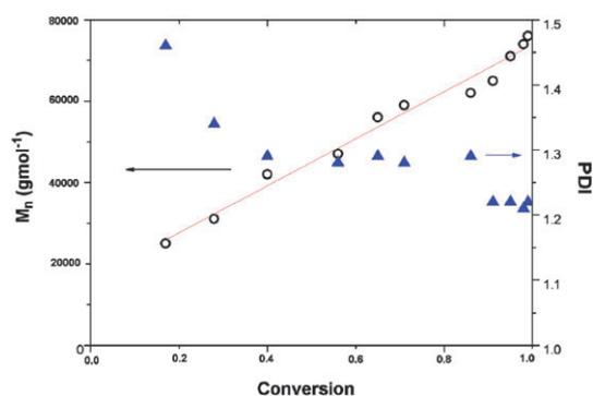
**Fig. 2** Molecular weight evolution and molecular weight distribution with monomer conversion for MMA showing excellent linear evolution and the expected narrowing of the PDI at higher conversions. Note also that the plot of molecular weight with conversion intercepts the y abscissa at 15 kDa; the molecular weight of the PFOMA surfactant as calculated by <sup>1</sup>H NMR.
