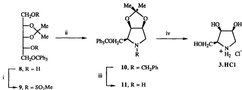
**Scheme 1.** i, excess MsCl, C<sub>5</sub>H<sub>5</sub>N, DMAP; ii, PhCH<sub>2</sub>NH<sub>2</sub>, 80°; iii, H<sub>2</sub>, Pd/C, EtOH; iv, TFA-H<sub>2</sub>O
