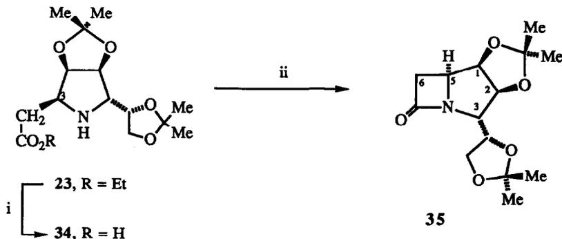
Scheme 6. i, K<sub>2</sub>CO<sub>3</sub>, MeOH, H<sub>2</sub>O; ii, Ph<sub>3</sub>P, (PyS)<sub>2</sub>, MeCN,  $\Delta$
