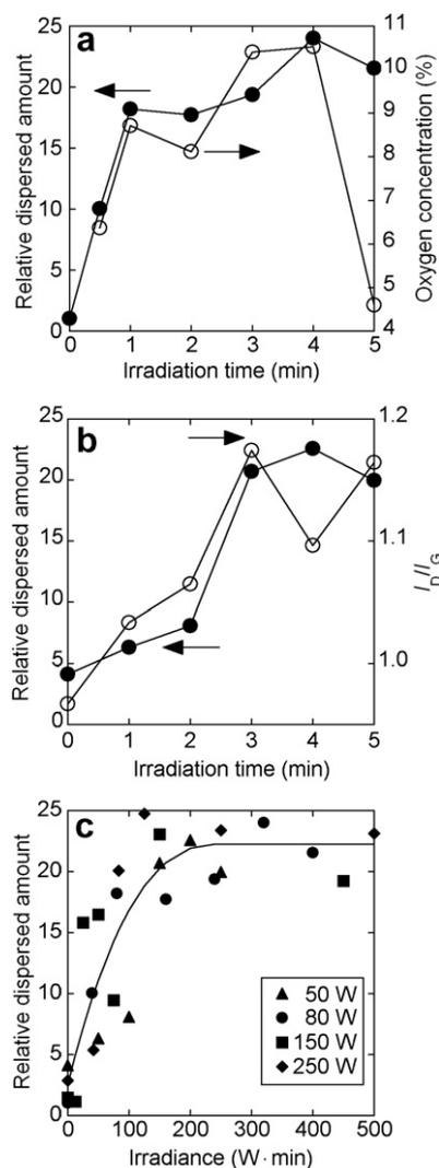
Fig. 1. (a) Relative dispersed amount of SWNHs in THF (closed circles) and oxygen concentration (open circles) for various irradiation times at 80 W. (b) Relative dispersed amount (closed circles) and the ratio of the band intensities (open circles) for various irradiation times at 50 W. (c) Relative dispersed amount plotted against irradiance for all conditions.
