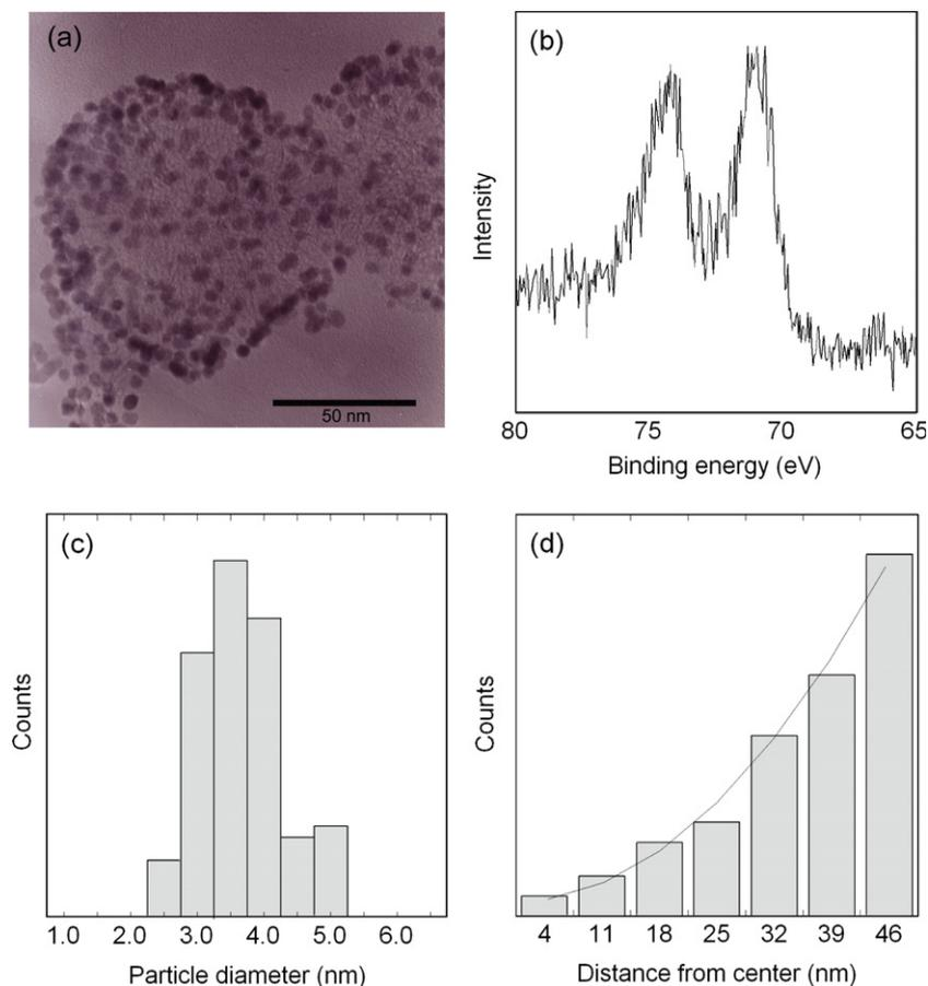
Fig. 2. (a) TEM image of Pt supporting SWNHs. (b) XPS spectrum of Pt supporting SWNHs. (c) Diameter distribution of Pt particles on SWNH. (d) A histogram of a number of Pt particles against the distance from the center of the SWNH imaged in TEM. The solid line is a parabolic function of the distance.
