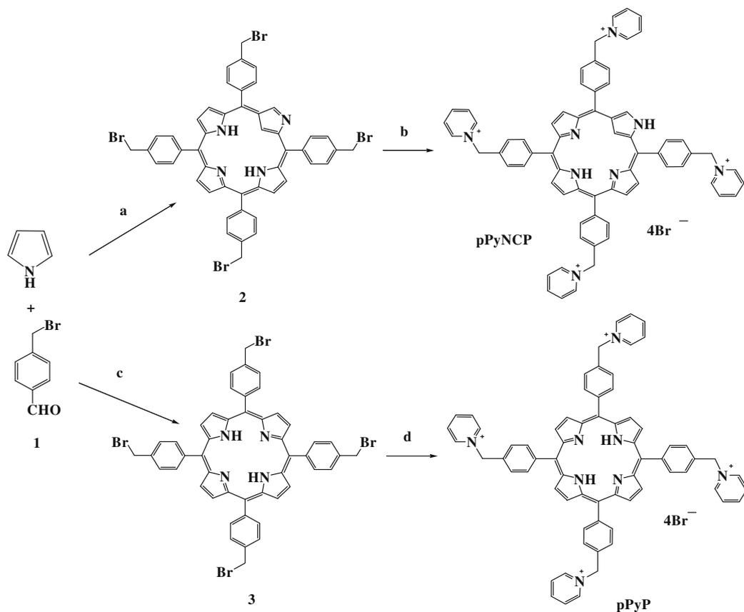
**Scheme 2.** Synthesis of pPyNCP. Reagents and conditions: (a) methanesulfonic acid (MSA), 2,3-dichloro-5,6-dicyano-*p*-benzoquinone (DDQ),  $\text{CH}_2\text{Cl}_2$ , 40 °C, 30 min; (b) pyridine, 40 °C, 7 days; (c)  $\text{BF}_3 \cdot \text{Et}_2\text{O}$ , chloranil,  $\text{CHCl}_3$ , 2 h; (d) pyridine, 110 °C, 1.5 h.
