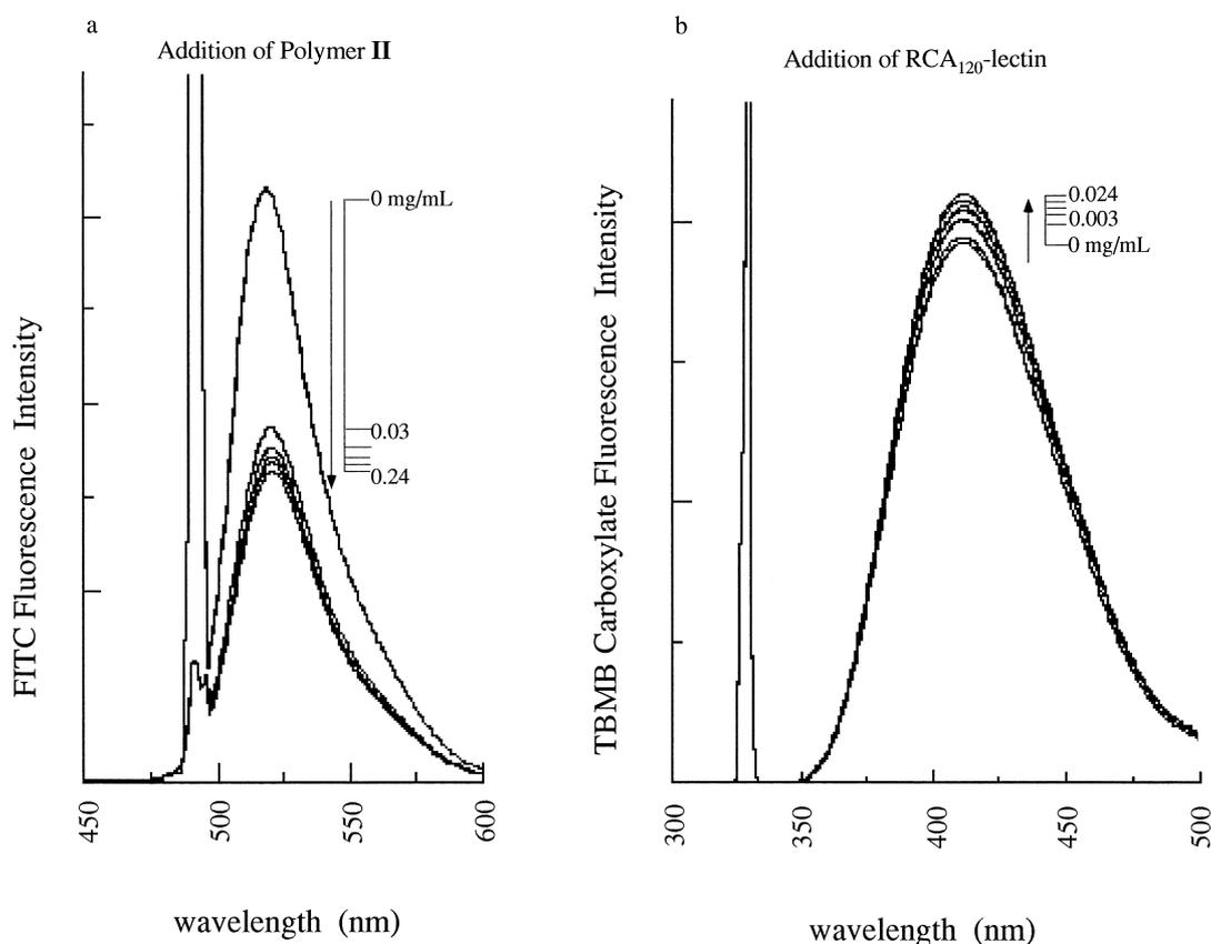
**Figure 2.** Fluorescence change of FITC (a) and TBMB carboxylate (b) chromophores upon the polymer II-RCA<sub>120</sub> lectin binding. In (a), an aliquot of a fluorescence polymer-II solution was added to the buffer solution of FITC-labeled lectin, while in (b), an aliquot of non-fluorescent lectin solution was added to the solution of TBMB-labeled polymer-II.
