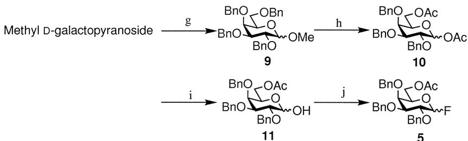
Reagents and Conditions: g) NaH, BnBr, DMF, 0°C, 12 h, 95%; h) Ac<sub>2</sub>O, H<sub>2</sub>SO<sub>4</sub>, 0°C, 2 h, 82%; i) 2-aminoethanol, DMSO, EtOAc, 48 h, 81%; j) HFPDEA, CH<sub>2</sub>Cl<sub>2</sub>, 0°C, 2 h, 95%
