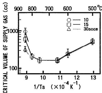
FIG. 2. Critical volume of supply gas for polycrystalline Si nucleation on SiO<sub>2</sub> vs substrate temperature. The critical volume of supply gas is equivalent to the product of the incubation time and the gas flow rate.
