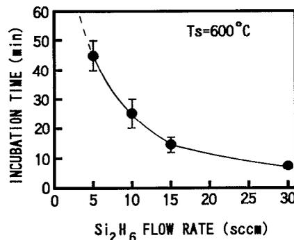
FIG. 1. Flow rate dependence of incubation time. When Si<sub>2</sub>H<sub>6</sub> was supplied for longer than the incubation time, polycrystalline Si was nucleated on the SiO<sub>2</sub>.
