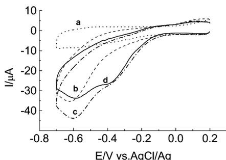
**Fig. 5** Cyclic voltammograms at the Pd nanoparticles electrodeposited on an Au electrode (potential cycling for hours) in 0.1 M KCl solution saturated with N<sub>2</sub> (a), (b) and air (c), (d) in the absence (a), (d) and the presence (b), (c) of 2.7 mM and 2.0 mM H<sub>2</sub>O<sub>2</sub>, respectively. Potential scan rate: 100 mV s<sup>-1</sup>.
