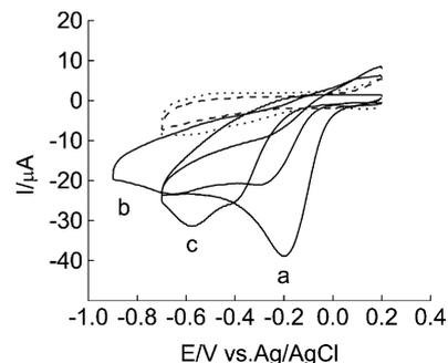
**Fig. 3** CVs obtained for the  $O_2$  reduction at: (a) freshly prepared Pd nanoparticles deposited on an Au electrode; (b) bulk Au electrode; (c) modified electrode of (a) after potential cycling for hours in air-saturated 0.1 M KCl solution. The dashed and dotted lines correspond to the bare and modified Au electrode, respectively, in  $N_2$ -saturated 0.1 M KCl solution. Potential scan rate:  $100 \text{ mV s}^{-1}$ .
