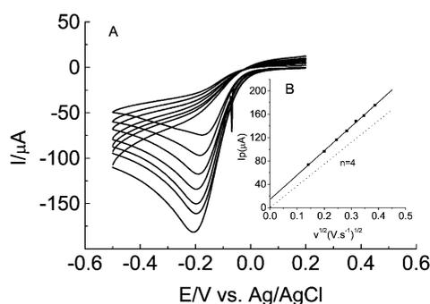
**Fig. 4** (A) Cyclic voltammograms of an  $O_2$ -saturated solution at 20, 40, 60, 80, 100, 120, and  $150 \text{ mV s}^{-1}$ . (B) Plot of the electrocatalytic dioxygen reduction peak current as a function of the square root of the scan rate (solid circles and line) and the calculated curve for the reaction with  $n = 4$  (dashed line). Electrolyte: 0.1 M KCl.
