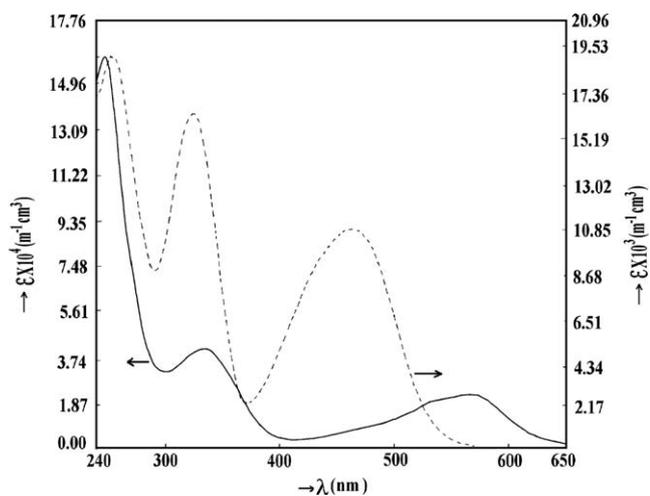
Fig. 1. UV-Vis spectra of  $HL^3$  (---) and  $(L^3)PdCl$  (—). The arrows indicate scales of the corresponding spectrum.
