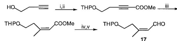
i. 3,4-DHP, PPTS, DCM, 25°C, 96%; ii. *n*-BuLi,  $\text{ClCOOMe}$ , THF, -60°C, 95%; iii.  $\text{CuI}$ , MeI,  $\text{Et}_2\text{O}$ , -78°C, 91%; iv. DIBAL,  $\text{Et}_2\text{O}$ , -78°C, 97%; v. TPAP, NMO, DCM, 93%
