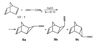
Attempts at using palladium compounds  $(Pd(OAc)_2, (PhCN)_2PdCl_2, Pd(acac)_2)$  as catalysts instead of CuCl failed because these compounds virtually do not decompose DAP at 20–25 °C.
