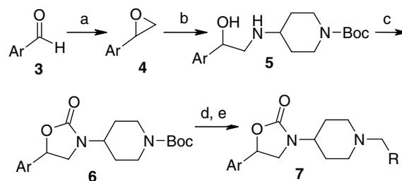
Scheme 1. Reagents and conditions: (a) Me<sub>2</sub>S, Me<sub>2</sub>SO<sub>4</sub>, NaOMe, CH<sub>3</sub>CN, rt; (b) 4-amino-piperidine-1-carboxylic acid *tert*-butyl ester, LiClO<sub>4</sub>, CH<sub>3</sub>CN, reflux; (c) 1,1-carbonyldiimidazole, 4-dimethylamino pyridine, CH<sub>2</sub>Cl<sub>2</sub>, rt; (d, e) 30% trifluoroacetic acid in CH<sub>2</sub>Cl<sub>2</sub>, rt; (e) RCHO, Na(OAc)<sub>3</sub>BH, CH<sub>2</sub>Cl<sub>2</sub>, rt.
